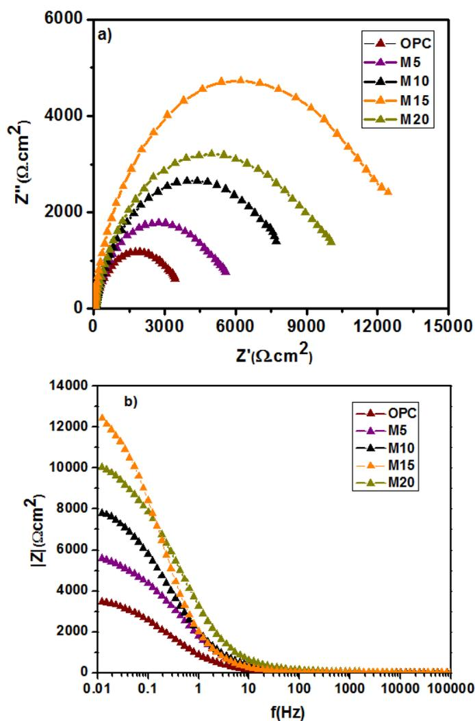
**Figure 2.** a) Nyquist and b) Bode plots of steel bars in concrete containing different metakaolin contents exposed to soil with a chloride concentration of 3%
