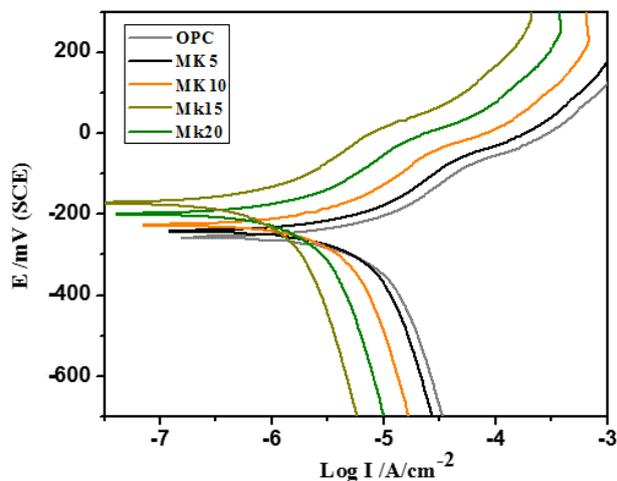
**Figure 4.** Polarization curves of steel bars in concrete containing different metakaolin contents exposed to soil with a chloride concentration of 3%
