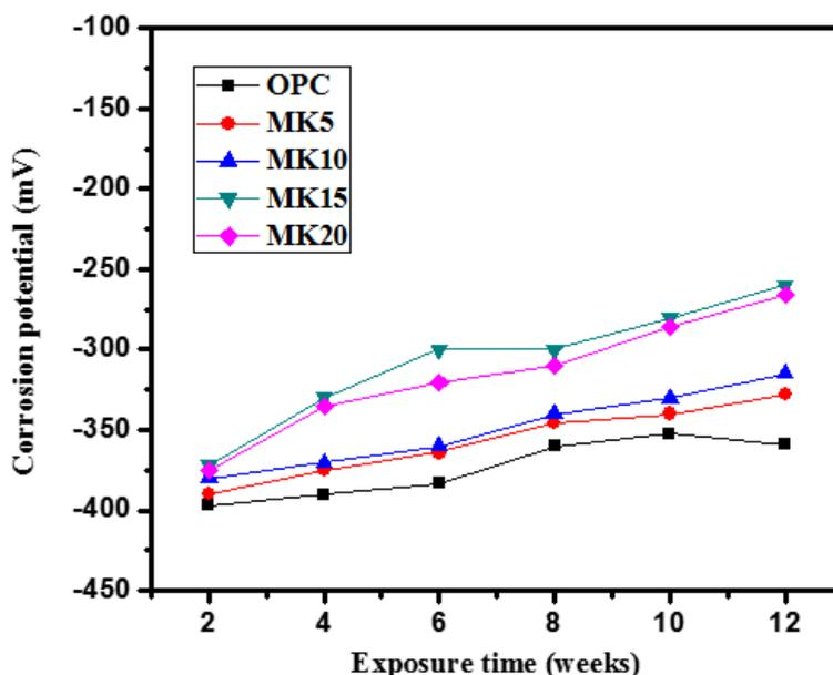
**Figure 1.** Corrosion potentials of carbon steel in concrete immersed into the soil containing 3 wt% chloride
