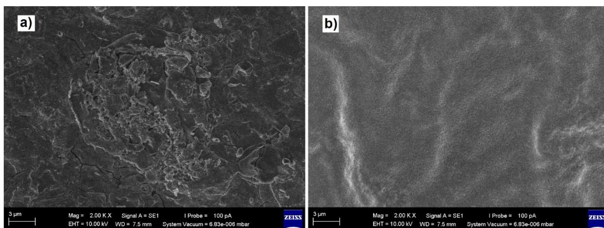
**Figure 5.** SEM images of concrete specimens, (a) OPC sample and (b) concrete sample containing 15 wt% metakaolin exposed to soil with a chloride concentration of 3% after 4 weeks
