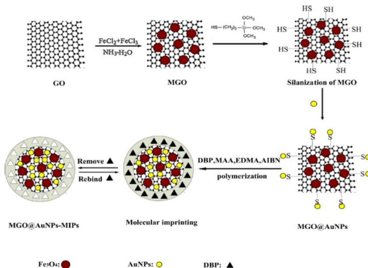
**Figure 2.** Preparation of magnetic graphene oxide MIP electrochemical sensor functionalized with gold nanoparticles. Reprinted with permission from reference [99].
