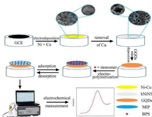
**Figure 1.** Preparation of BPS MIP electrochemical sensor modified by hollow nickel nanospheres coated with graphene quantum dots. Reprinted with permission from reference [98].
