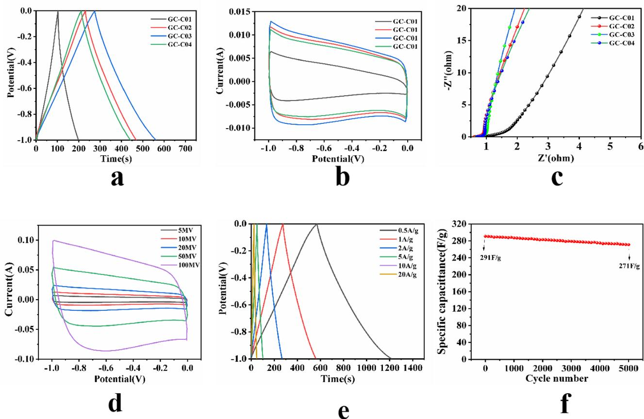
**Figure 5.** Electrochemical performance of the samples measured in a three-electrode system. (a)GCD curves of all the samples at the current density of 1A/g; (b)CV curves of all the samples at a scan rate of 10mV/s; (c)EIS of all the samples; (d)CV curves for GC-C03 at scan rates ranging from 5mV/s to 100mV/s;(e) GCD curves of GC-C03 at different current densities; (f)GC-C03 in specific capacitance retention rates at the current density of 1A/g after 5000 cycles.
