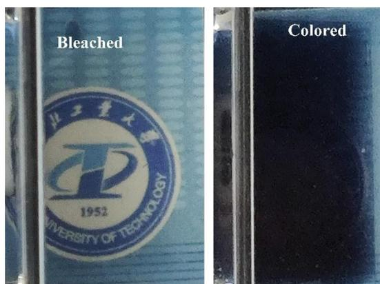
**Figure 5.** Picture of the bleached state of the film and the colored state at -1.6 V
