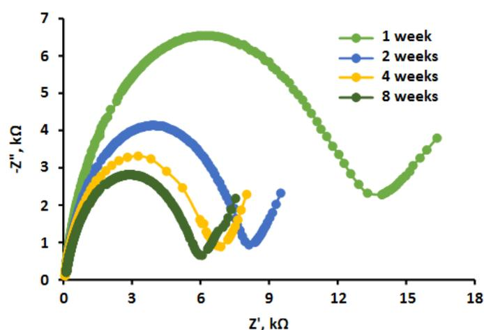
**Figure 5.** Nyquist diagrams of the 10MIO specimen immersed in 3.5wt% NaCl solution in different exposure times at room temperature
