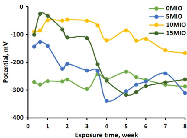
**Figure 2.** OCP versus exposure time of the coated steel reinforced concrete with different ER coatings containing MIO
