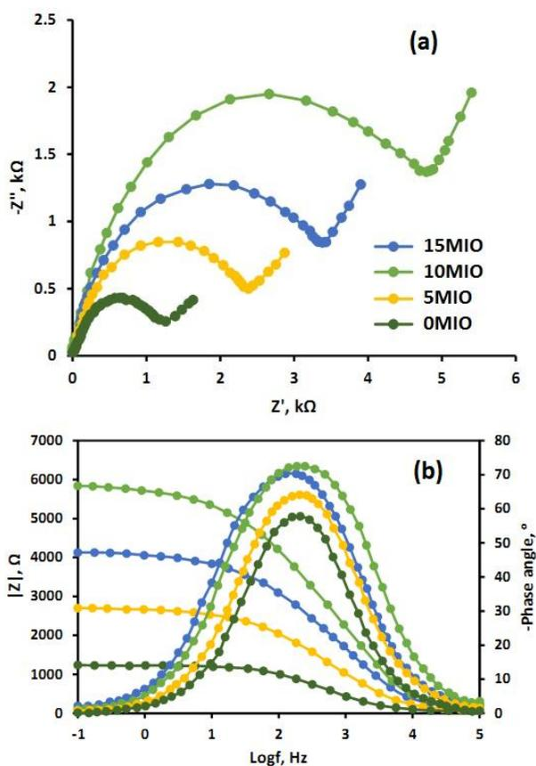
**Figure 3.** (a) Nyquist and (b) bode diagrams of the coated steel reinforced concrete with different ER coatings containing MIO immersed in 3.5wt% NaCl media after 8 weeks
