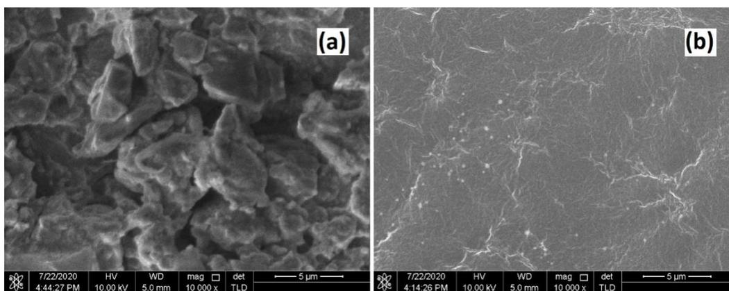
**Figure 7.** Surface morphology of steel rebars with various epoxy coatings (a) MIO-free, (b) 10-MIO samples immersed to 3.5wt% NaCl media for 4 weeks
