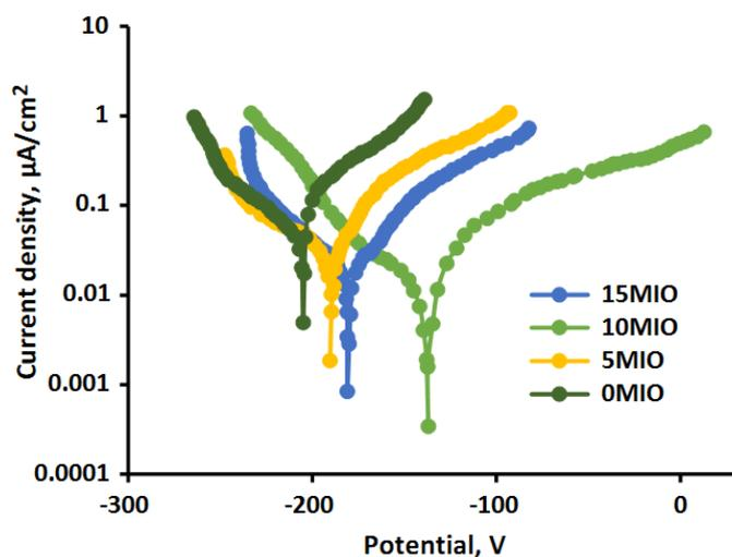
**Figure 6.** Polarization diagrams of steel rebars coated by ER containing the various concentrations of MIOs exposed to 3.5wt% NaCl media for 4 weeks at room temperature
