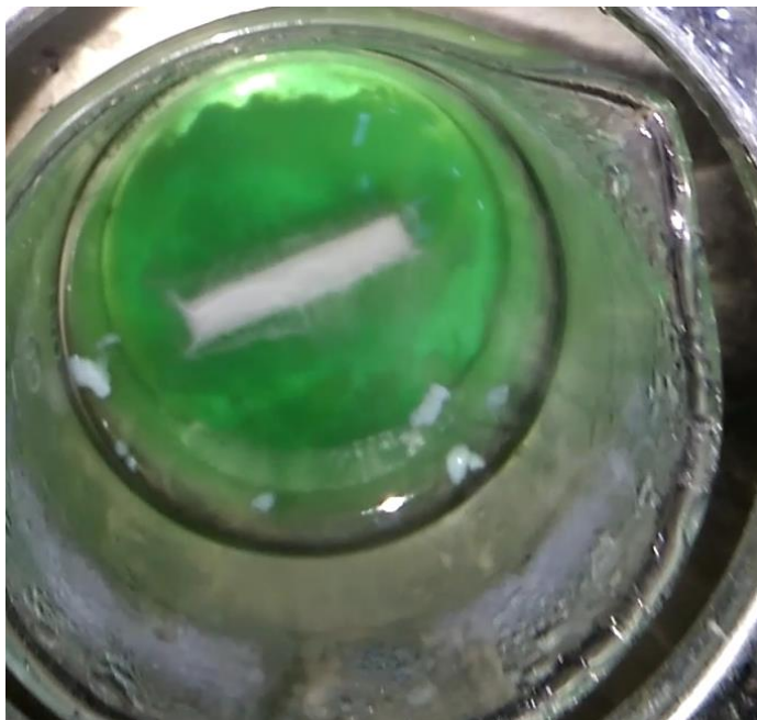
Figure 1. Nickel composite metallic particles floated on the electrolyte
