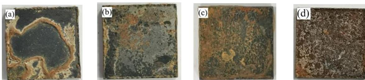
**Figure 10.** Macro-images of the corrosion of Q235 steel in 0%(a), 0.3%(b), 1.3%(c), and 2.3%(d) sodium chloride silt soil for 60 days
