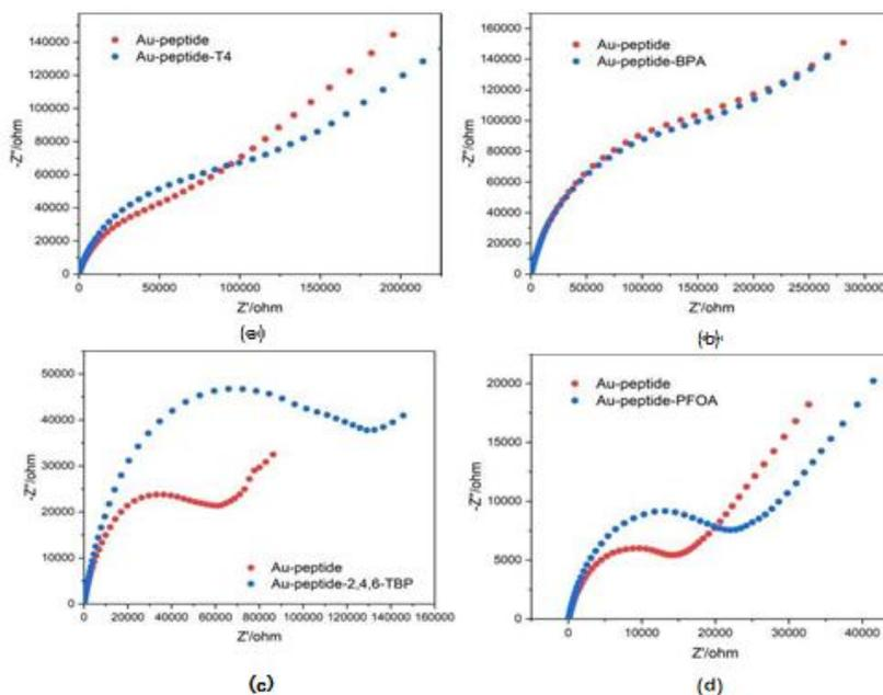
**Figure 3.** Impedance changes following absorption onto the Au-peptide 4 electrode for (a) T4 positive control (b) BPA negative control and the known TDCs (c) 2,4,6-TBP and (d) PFOA.
