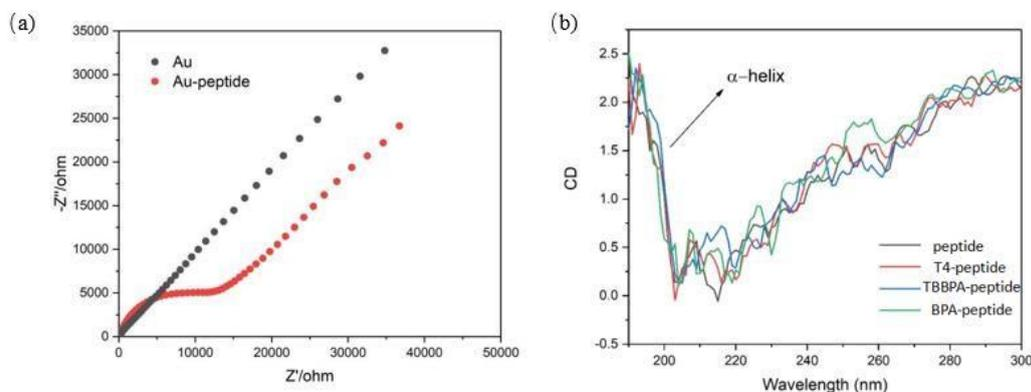
**Figure 2.** (a). Au electrode resistance measurements before and after peptide modification (b). CD analysis of peptide 4 in the presence and absence of the indicated compounds
