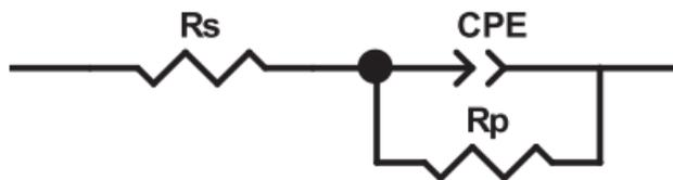
**Figure 6.** Equivalent circuit model for EIS
