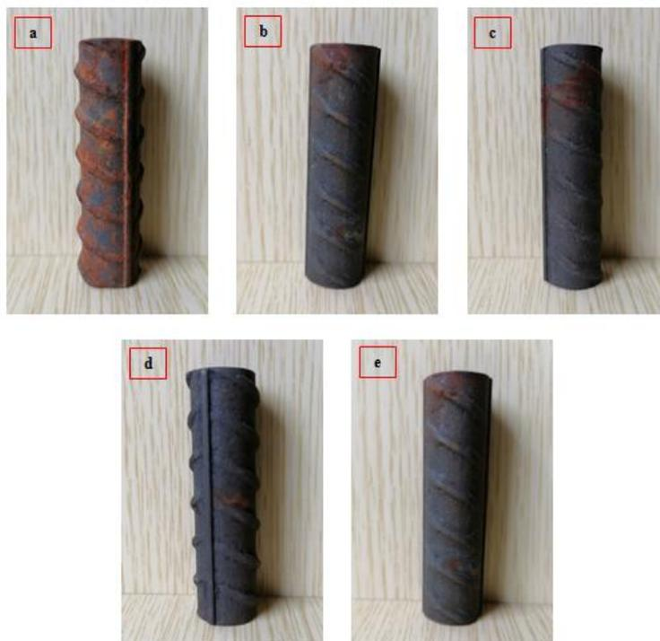
**Figure 6.** Appearance of different rebar steel samples after 48h salt spray testing in 5% sodium chloride solution; a-conventional rebar steel sample; b-phosphatized rebar steel sample; c-phosphatized rebar steel sample after sealing with 4 g/L sodium silicate; d-phosphatized rebar steel after sealing with 10 g/L sodium silicate; e-phosphatized rebar steel after sealing with 16 g/L sodium silicate (auto focus with double magnification)
