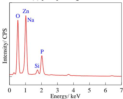
(b) phosphating film after sealing with 10 g/L sodium silicate
