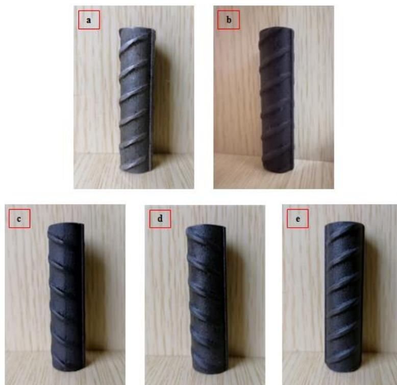
**Figure 1.** Appearance of different rebar steel samples; a-conventional rebar steel sample; b-phosphatized rebar steel sample; c-phosphatized rebar steel sample after sealing with 4 g/L sodium silicate; d-phosphatized rebar steel after sealing with 10 g/L sodium silicate; e-phosphatized rebar steel after sealing with 16 g/L sodium silicate; (auto focus with double magnification)
