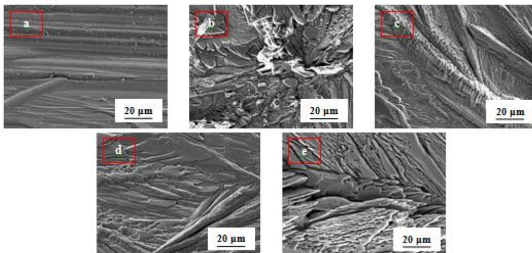
**Figure 2.** Surface morphology of rebar steel, phosphating film and phosphating film after sealing a-rebar steel sample; b-phosphating film; c-phosphating film after sealing with 4 g/L sodium silicate; d-phosphating film after sealing with 10 g/L sodium silicate; e-phosphating film after sealing with 16 g/L sodium silicate (sample size 6 mm×6 mm×1 mm, magnification 1500 times, accelerating voltage 10 kV)
