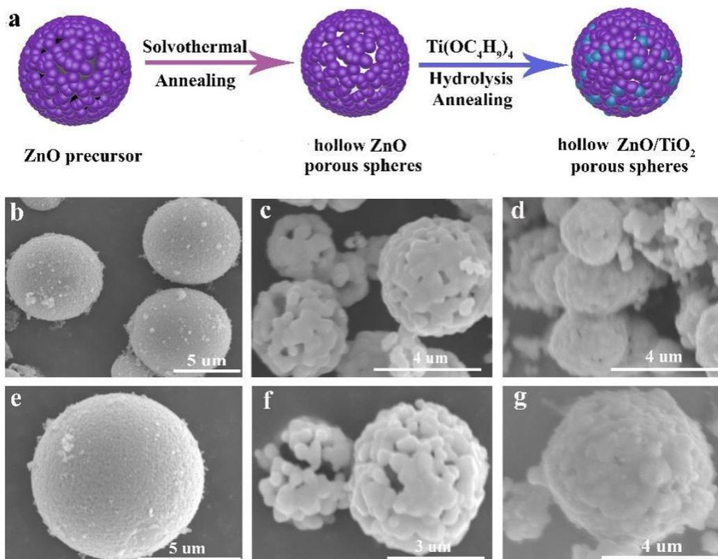
**Figure 1.** (a) Schematics fabrication process of hollow ZnO/TiO<sub>2</sub> composite spheres, SEM images of (b, e) ZnO precursor, (c, f) hollow ZnO porous spheres, (d, g) hollow ZnO/TiO<sub>2</sub> composite spheres.
