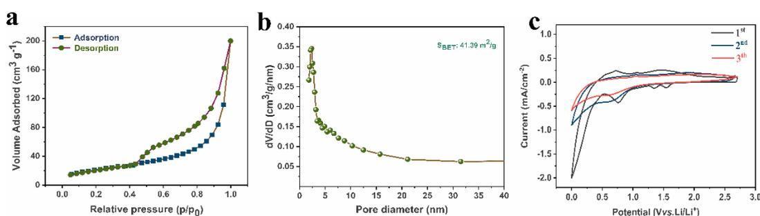
**Figure 4.** (a) Nitrogen adsorption-desorption isotherms. (b) pore size distribution of hollow ZnO/ $\text{TiO}_2$  composite spheres. (c) CV curves of hollow ZnO/ $\text{TiO}_2$  composite spheres.
