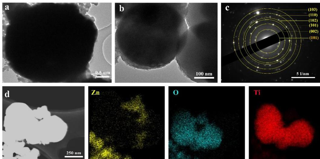
**Figure 2.** TEM and HRTEM images of hollow ZnO/TiO<sub>2</sub> composite spheres: (a) TEM image, (b) HRTEM image, (c) electron diffraction spectra, (d) EDX elemental mapping images
