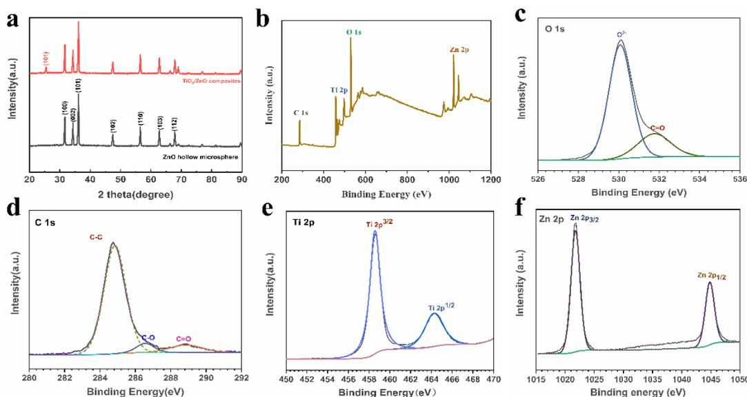
**Figure 3.** (a) XRD patterns of porous hollow ZnO spheres and hollow ZnO/TiO<sub>2</sub> composite spheres. XPS spectra of hollow ZnO/TiO<sub>2</sub> composite spheres: (b) survey spectra, (c) O 1s core-level spectra, (d) C 1s core-level spectra, (e) Ti 2p core-level spectra, (f) Zn 2p core-level spectra.
