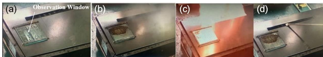
Figure 8. Power battery box thermal runaway suppression experiment. (a) Before thermal runaway. (b) When thermal runaway occurs. (c) Open flame ignition experiment. (d) After the fire extinguishing agent has been sprayed.
