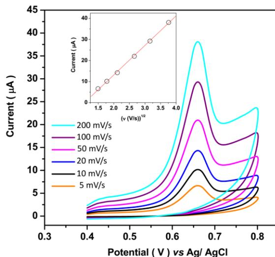
**Figure 5.** CV curves of MIP/NiO NPs/GCE at the potential range from 0.40 V to 0.80 V in 0.1 M PBS (pH 7.0) containing 70  $\mu\text{M}$  PEN solution at scanning rate from 5 to 200 mV/s.
