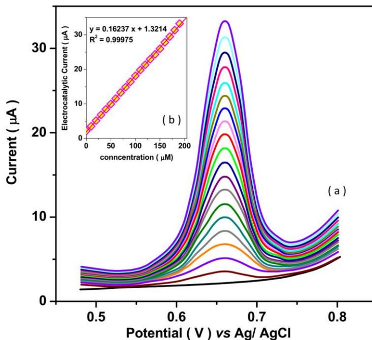
**Figure 6.** (a) The DPV responses of MIP/NiO NPs/GCE at the potential range from 0.48 V to 0.80 V with a scanning rate of 20 mV/s to each injection of 10  $\mu\text{M}$  PEN solutions in electrochemical cell containing 0.1 M PBS (pH 7.0); (b) calibration plot.
