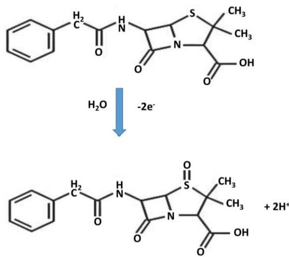
**Figure 4.** The suggested mechanism of electro-oxidation of PEN [57].
