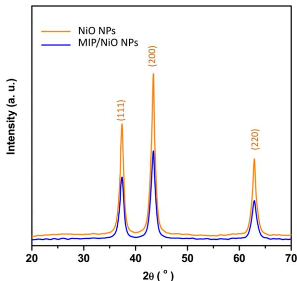
**Figure 2.** Results of structural characterization of powders of NiO NPs and MIP/NiO NPs using X-ray diffraction technique.
