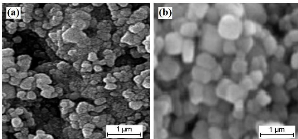
**Figure 1.** SEM micrographs of the morphological structures of (a) NiO NPs and (b) MIP/NiO NPs modified GCE.
