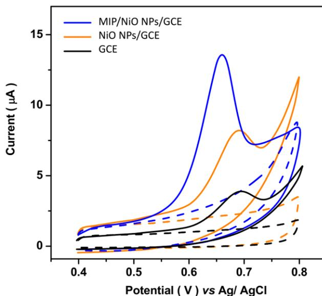
**Figure 3.** The CV curves of unmodified GCE, NiO NPs/GCE and MIP/NiO NPs/GCE at the potential range from 0.40 V to 0.80 V at scanning rate of 20 mV/s in 0.1 M PBS (pH 7.0) in absence (dashed line) and presence (solid line) of 70  $\mu\text{M}$  PEN solution.
