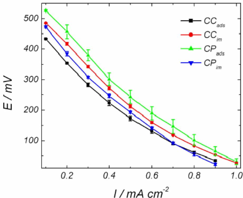
**Figure 1** - Current density versus cell potential for a PEMFC. Anode:  $0,4\ mg\ Pt\ cm^{-2}$ , cathode: adsorbed ( $CC_{ads}$ ) and immobilized ( $CC_{im}$ ) peroxidase extract on carbon cloth, and adsorbed ( $CP_{ads}$ ) and immobilized ( $CP_{im}$ ) peroxidase extract on carbon powder. The error bars present the deviation observed for independent sets of experiments. Temperature  $25^{\circ}C$ .
