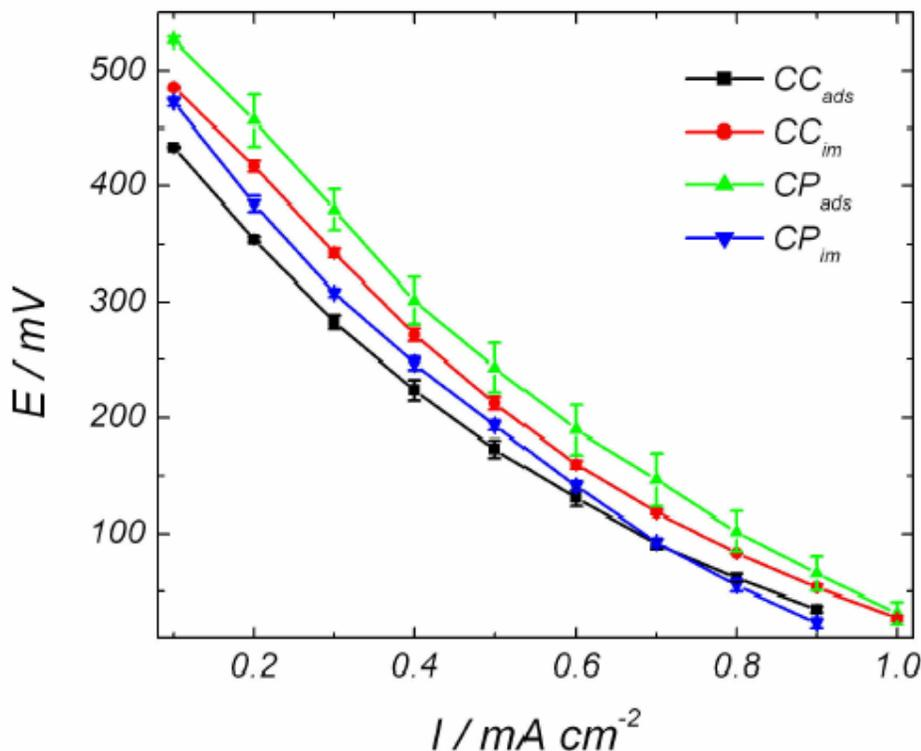
**Figure 1** - Current density versus cell potential for a PEMFC. Anode:  $0,4 \text{ mg Pt cm}^{-2}$ , cathode: adsorbed ( $CC_{ads}$ ) and immobilized ( $CC_{im}$ ) peroxidase extract on carbon cloth, and adsorbed ( $CP_{ads}$ ) and immobilized ( $CP_{im}$ ) peroxidase extract on carbon powder. The error bars present the deviation observed for independent sets of experiments. Temperature  $25^{\circ}\text{C}$ .
