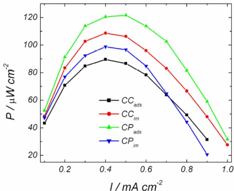
**Figure 2** - Plots of power density versus cell current density for the four different configurations displayed in Figure 1.
