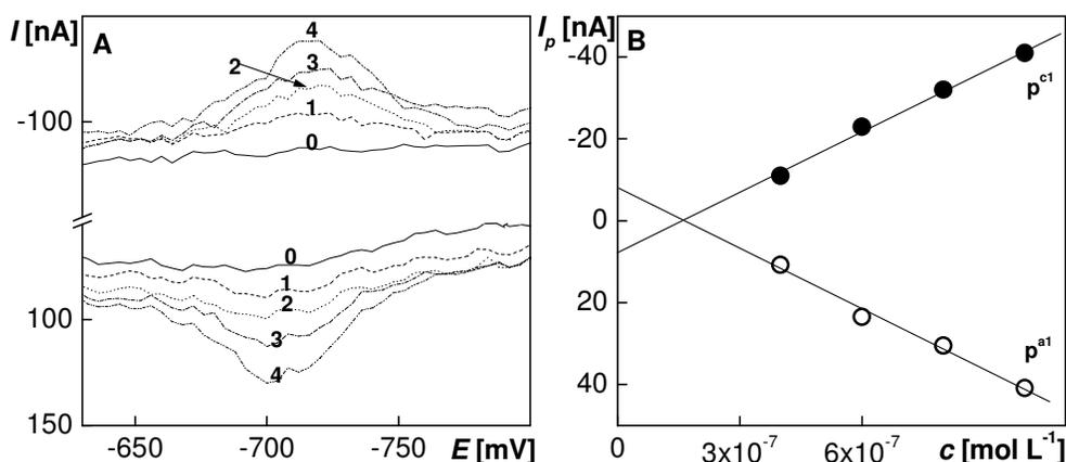
**Figure 11.** Cyclic voltammograms of TPPS4 in BR buffer, pH 7.0, scan rate  $500 \text{ mV s}^{-1}$ ;  $c$  (TPPS4) = 0 (0),  $4 \cdot 10^{-7}$  (1),  $6 \cdot 10^{-7}$  (2),  $8 \cdot 10^{-7}$  (3),  $10 \cdot 10^{-7}$  (4)  $\text{mol L}^{-1}$  (A) and corresponding calibration dependence (B).
