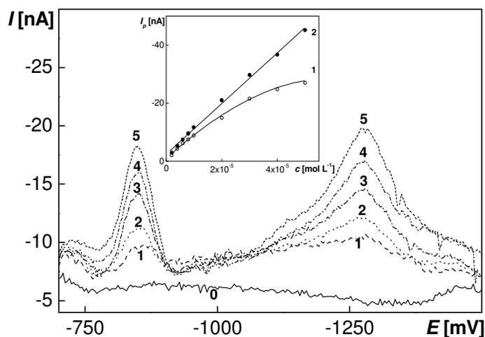
**Figure 6.** DP polarograms of TPPS4 in BR buffer pH 10; analyte concentration: 0 (0),  $2 \cdot 10^{-6}$  (1),  $4 \cdot 10^{-6}$  (2),  $6 \cdot 10^{-6}$  (3),  $8 \cdot 10^{-6}$  (4),  $10 \cdot 10^{-6}$  (5)  $\text{mol L}^{-1}$ . Inset is the calibration dependence of the first (1,  $\circ$ ) and the second (2,  $\bullet$ ) peak.
