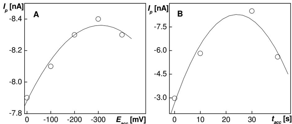
**Figure 7.** Dependence of the height of the AdSV peak ( $I_p$ ) of TPPS4 ( $c = 1 \cdot 10^{-6} \text{ mol L}^{-1}$ ) on potential of accumulation  $E_{acc}$  (A;  $t_{acc} = 30 \text{ s}$ ) and the time of accumulation  $t_{acc}$  (B;  $E_{acc} = -300 \text{ mV}$ ) in BR buffer pH 5.
