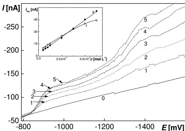
**Figure 4.** DC tast polarograms of TPPS4 in BR buffer, pH 10, analyte concentration: 0 (0),  $1 \cdot 10^{-5}$  (1),  $2 \cdot 10^{-5}$  (2),  $3 \cdot 10^{-5}$  (3),  $4 \cdot 10^{-5}$  (4),  $5 \cdot 10^{-5}$  (5) mol L<sup>-1</sup>. Inset is the calibration dependence of the first (1,  $\circ$ ) and the second (2,  $\bullet$ ) wave.
