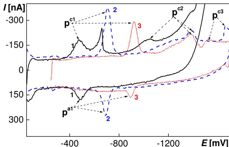
**Figure 9.** Selected cyclic voltammograms of TPPS4 ( $c = 1 \cdot 10^{-5}$  mol L<sup>-1</sup>) at HMDE in BR buffer, pH: 4.0 (1; —), 7.0 (2; ----), and 10.0 (3; .....). The first scan presented, scan rate  $500 \text{ mV s}^{-1}$ .
