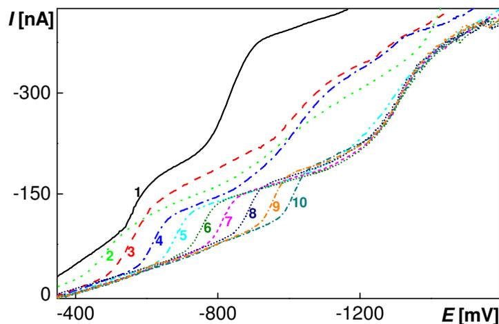
**Figure 2.** DC tast polarograms of TPPS4 ( $c = 5 \cdot 10^{-5} \text{ mol L}^{-1}$ ) in BR buffer of pH 2 (1), 4 (2), 5 (3), 6 (4), 7 (5), 8 (6), 9 (7), 10 (8), 11 (9), 12 (10).
