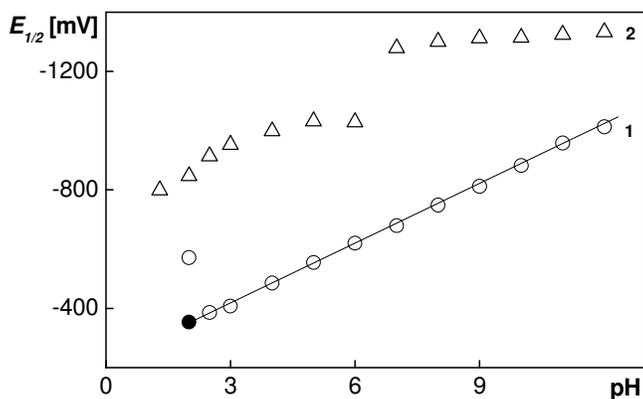
**Figure 3.** Dependence of the half wave potential  $E_{1/2}$  of the first (1) and second (2) wave of TPPS4 ( $c = 5 \cdot 10^{-5}$  mol L<sup>-1</sup>) on pH of BR buffer (pH 2-12,  $\circ$ ) and  $0.01$  mol L<sup>-1</sup> Na<sub>2</sub>HPO<sub>4</sub> (pH 2,  $\bullet$ ) measured by DC tast polarography.
