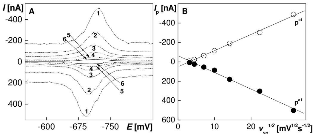
**Figure 10.** Cyclic voltammograms of TPPS4 ( $c = 1 \cdot 10^{-5}$  mol L<sup>-1</sup>) in BR buffer pH 7.0, scan rate  $v_{sc} = 1000$  (1), 500 (2), 200 (3), 100 (4), 50 (5) and 20 (6)  $\text{mV s}^{-1}$  (A) and corresponding dependence of the peak height  $I_p$  for the cathodic peak  $p^{c1}$  and anodic peak  $p^{a1}$  on the square root of the scan rate  $v_{sc}^{1/2}$  (B). The first scan presented and evaluated.
