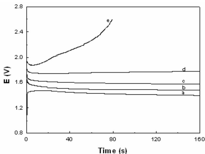
**Figure 1.** Chronopotentiometric curves obtained during galvanostatic polymerization of CIT in [BMIM]PF<sub>6</sub> at the different current densities: (a) 0.09 mA cm<sup>-2</sup> (b) 0.18 mA cm<sup>-2</sup> (c) 0.36 mA cm<sup>-2</sup> (d) 0.72 mA cm<sup>-2</sup> (e) 1.25 mA cm<sup>-2</sup>
