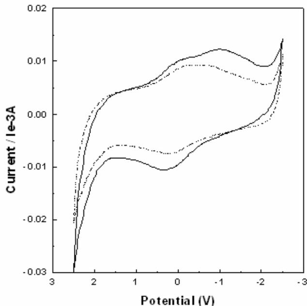
**Figure 6.** Cyclic voltammogram of POcT based solid ECD as a function of repeated scans at 500mV / s: (—) 1<sup>st</sup> cycle and (---) 1000<sup>th</sup> cycle
