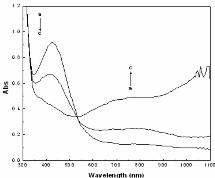
**Figure 5.** Spectroelectrochromistry of POcT based solid ECD as a function of applied voltage: -2.0 V (a) 1.8 V and (c) 2.2 V
