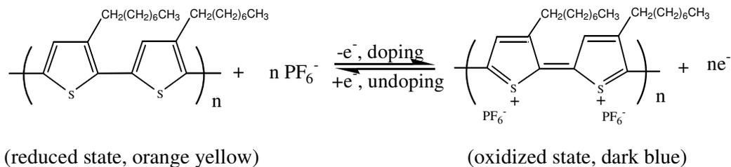
**Figure 4.** Electrochromism for POcT. The orange yellow (undoped) form undergoes reversible oxidation to the dark blue (doped) form, with insertion of charge-compensating anions (PF<sub>6</sub><sup>-</sup>)
