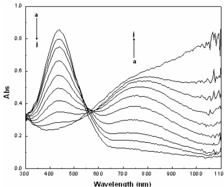
**Figure 3.** Spectroelectrochemistry of POcT (synthesized in [BMIM]PF<sub>6</sub> galvanostat on ITO) in pure ionic liquid [BMIM]PF<sub>6</sub>. Spectra were recorded at the following potentials: a: 0.4, b: 0.8, c: 0.9, d: 1.0, e: 1.1, f: 1.2, g: 1.3, h: 1.4, i: 1.5, j: 1.6V vs Ag/AgCl.
