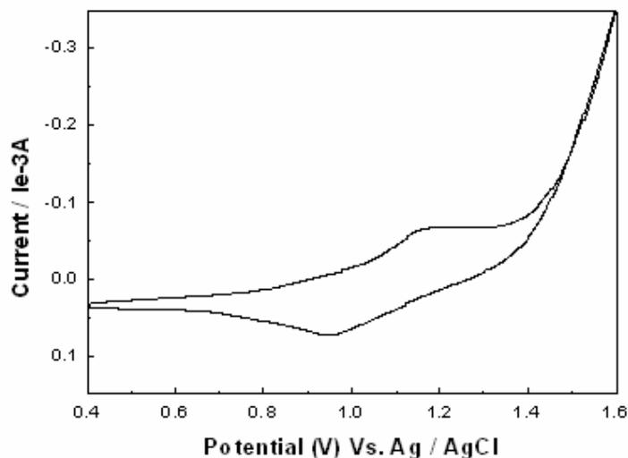
**Figure 2.** Electrochemical characterization of the POcT film in pure [BMIM]PF<sub>6</sub>. The scan rate was  $50 \text{ mV s}^{-1}$
