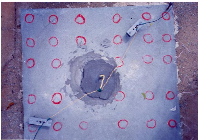
Slab with chloride and zinc overlay with cathodic protection
