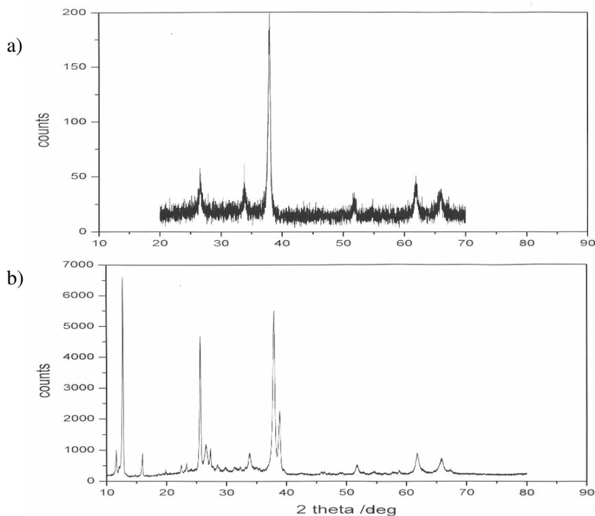
**Figure 1.** XRD patterns of (a) as-deposited and (b) air-annealed samples. Annealing temperature and time were  $450^\circ\text{C}$  and 1 hr. respectively.
