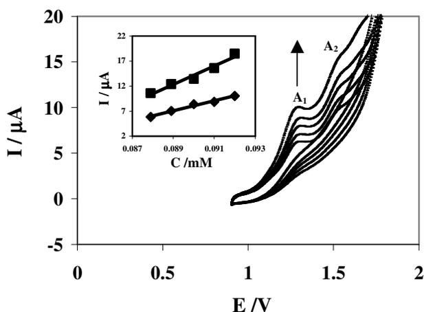
**Figure 2.** The cyclic voltammograms of compound **1** in 0.10 M TEAP+ DMF solutions at different concentrations; 0.088, 0.089, 0.90, 0.091, 0.092 mM, scan rate 100mVs<sup>-1</sup>.
