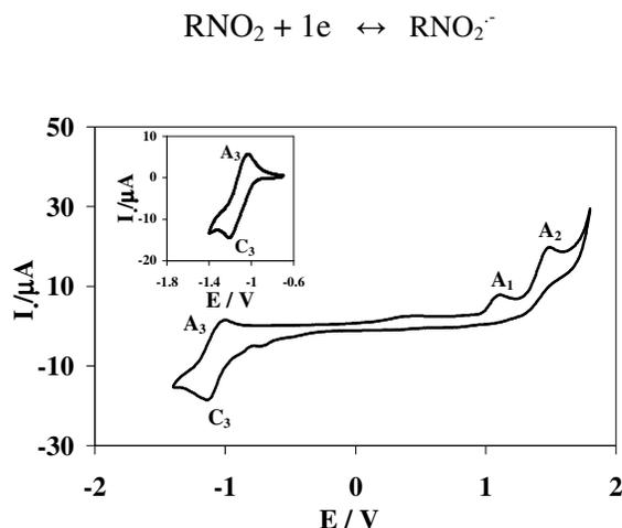
**Figure 4.** The cyclic voltammogram of **2** at wide range of -1.40 to 1.80 V, 0.10 M TEAP+ DMF solution, scan rate: 100  $\text{mVs}^{-1}$ . Inset: The cyclic voltammogram of **2** at potential range -1.40 to -0.70 V.
