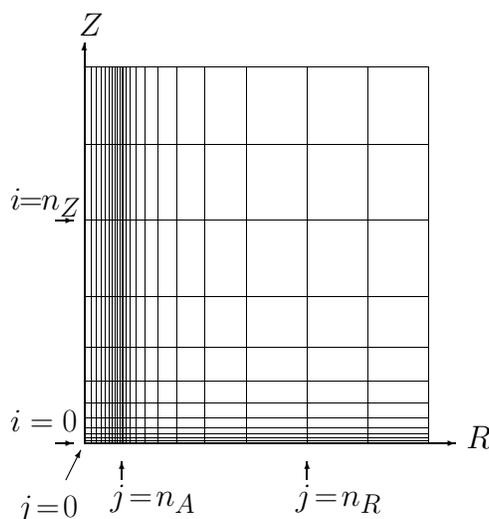
**Figure 3.** Discrete grid representing the cylindrical disk system
