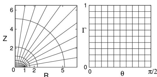
**Figure 4.** Discrete grid in transformed coordinates on the right with equal intervals, and the equivalent grid in cylindrical coordinates on the left (some grid lines are outside the picture in  $(R,Z)$ )
