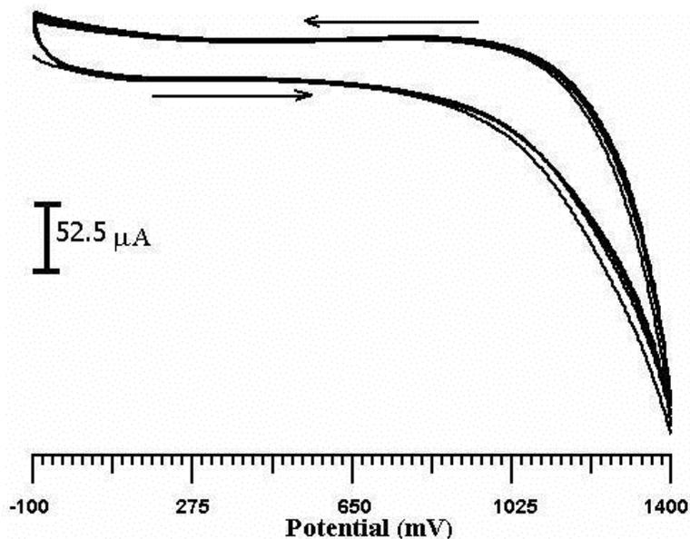
**Figure 1.** Cyclic voltammograms for 1mM DL-alanine recorded with bare CPE in 0.2 M ABS (pH 7.0) scan rate 50 mV/s
