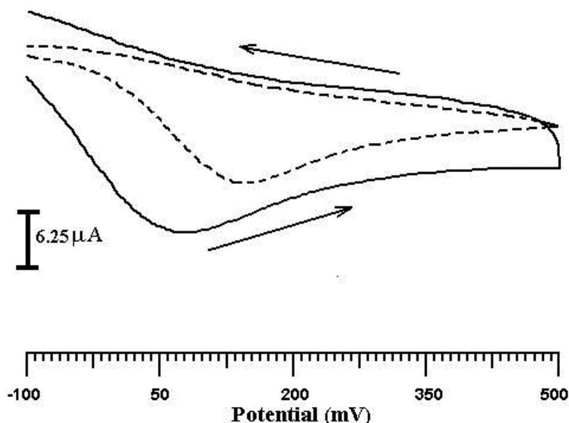
**Figure 3.** Cyclic voltammograms obtained for the oxidation of 1 mM AA at poly (alanine) MCPE (solid line curve) and bare CPE (dashed line curve) at scan rate 50mV/s
