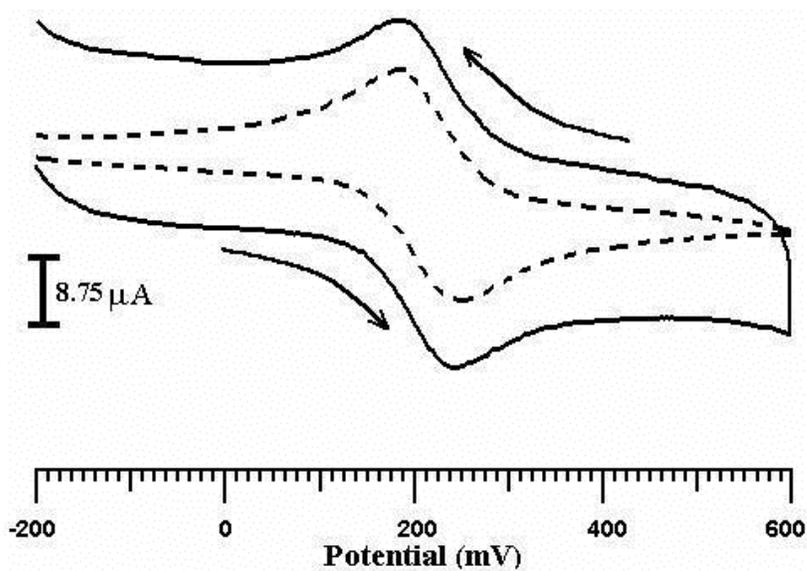
**Figure 2.** Cyclic voltammograms obtained for the electrochemical response of 1 mM  $\text{K}_4 [\text{Fe} (\text{CN})_6]$  at poly (alanine) modified electrode (solid line curve) and bare CPE (dashed curve line) in 1 M KCl. Scan rate 50 mV/s
