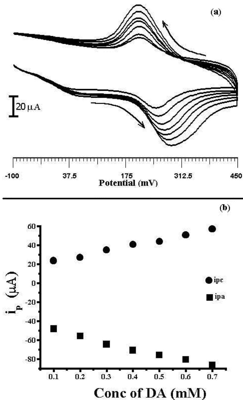
**Figure 6.** (a) Cyclic voltammograms obtained at the poly (alanine) MCPE in 0.2 M ABS pH 7.0 containing 1mM AA and DA with different concentrations (a) 0.1 (b) 0.2 (c) 0.3 (d) 0.4 (e) 0.5 (f) 0.6 (g) 0.7 mM at a scan rate of 50 mV/s (b) plot of redox peak current of DA verses concentration.
