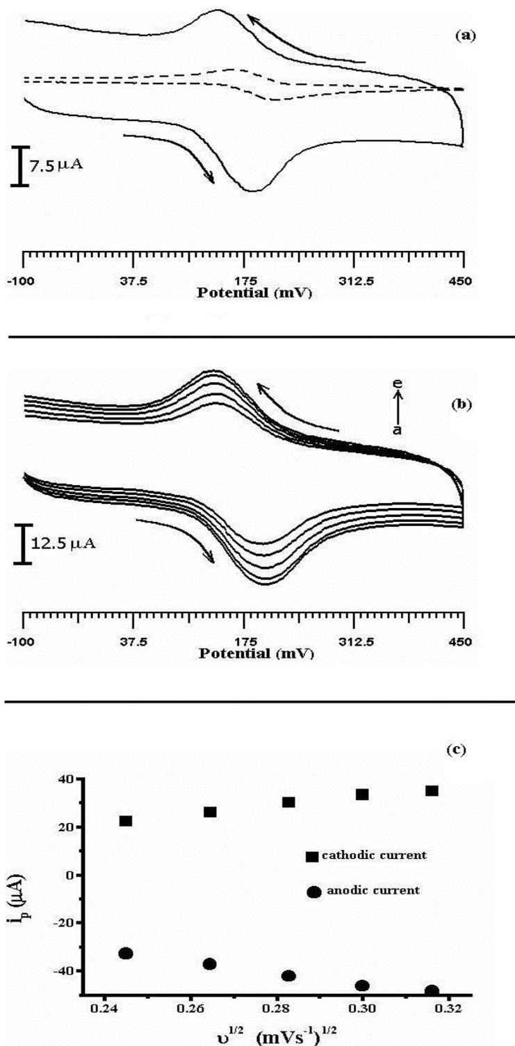
**Figure 4.** (a) Cyclic voltammograms for the oxidation of 0.1 mM DA obtained at the poly (alanine) MCPE (solid line curve) and bare CPE (dashed line curve) Scan rate 50 mV/s, 0.2 M ABS (pH. 7.0) (b) Cyclic voltammograms of 0.1 mM DA on the Poly (alanine) modified CPE at different scan rates (a – e: 60, 70, 80, 90,100 mV/s) in 0.2 M ABS (pH.7.0) and (c) is the plot of the redox peak current versus the square root of scan rate.
