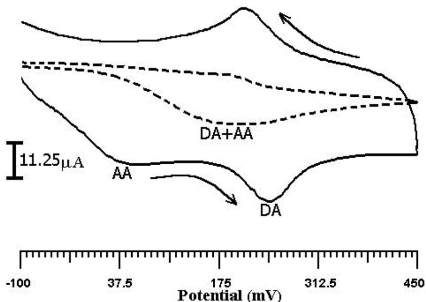
**Figure 5.** Cyclic voltammograms obtained at bare CPE (dashed line curve) and poly (alanine) MCPE (solid line curve) in 0.2 M ABS (pH 7.0) containing a mixture of 0.1 mM DA and 1 mM AA. Scan rate 50 mV/s.
