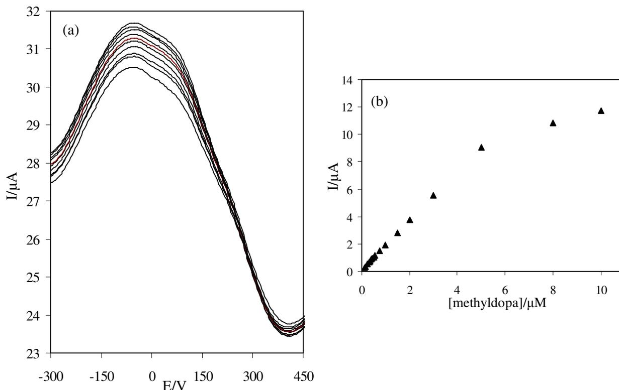
**Figure 6.** (a) Differential pulse voltammograms corresponding to the electrochemical responses of TR/SWCNTs/GC electrode, generated by different concentrations of methyl dopa in PBS from inner to outer; 0, 0.1, 0.14, 0.22, 0.3, 0.35, 0.4, 0.45, 0.5 and 0.55  $\mu\text{M}$ . The step potential and modulation amplitude values of 5 mV and 25 mV, respectively. (b) Calibration curve corresponding to the electrochemical analysis of DPVs for various concentrations of methyl dopa.
