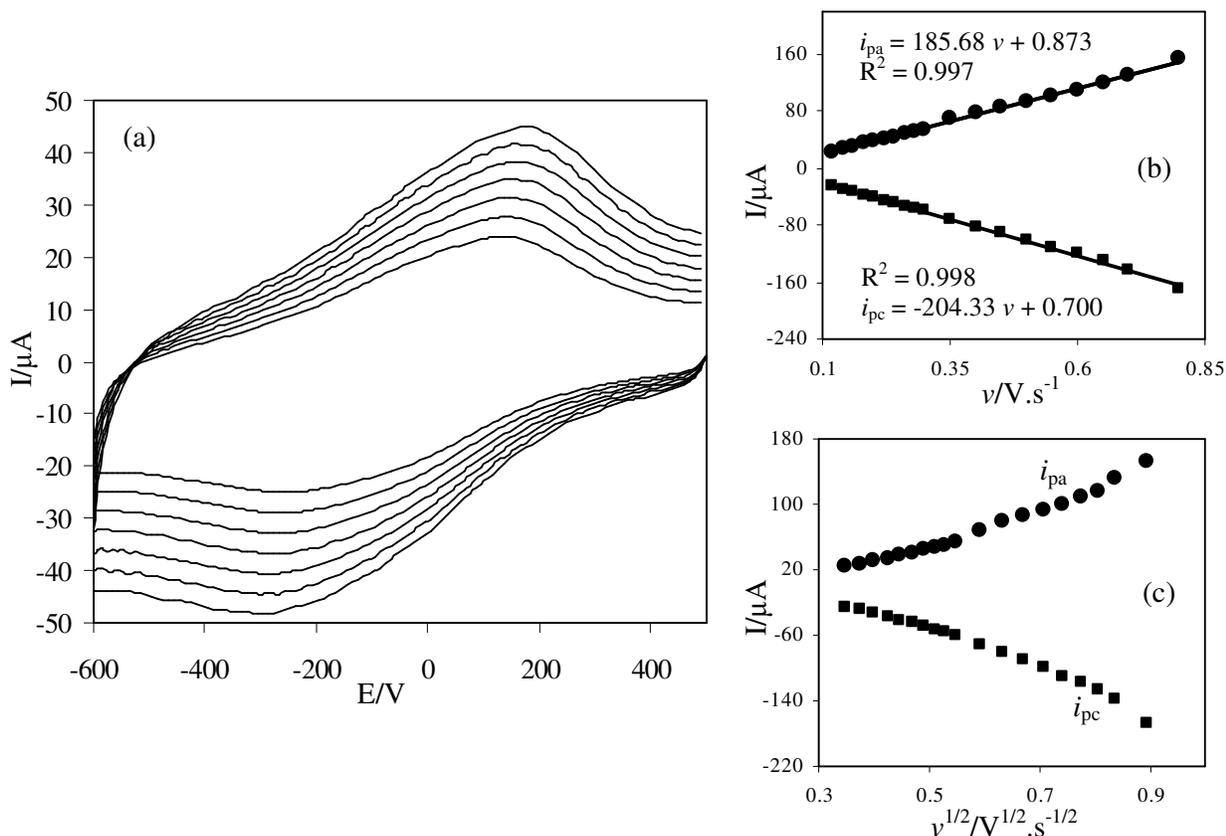
**Figure 4.** (a) The CVs of TR/SWCNTs/GC electrode in PBS at various scan rates, from inner to outer; 120, 140, 160, 180, 200, 220 and 240 mV/s. The relationship between the peak currents ( $i_{pa}$ ,  $i_{pc}$ ) vs. (b) the scan rates and (c) the square root of scan rates.
