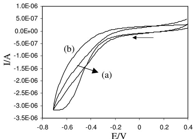
**Figure 2.** Comparative voltammograms of GC electrode; (a) in PBS, (b) in PBS containing 3 mg/mL tyrosinase, scan rate; 40 mV/s.
