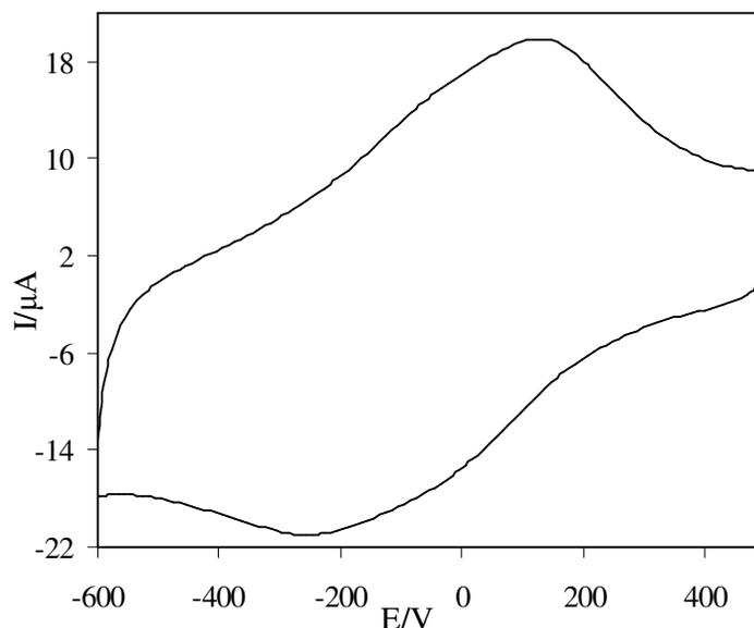
**Figure 3.** The recorded cyclic voltammogram in PBS for TR/SWCNTs/GC electrode, scan rate; 100 mV/s.
