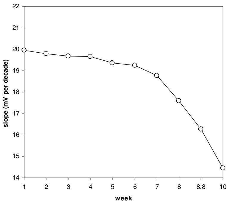
**Figure 3.** The lifetime of the Ho<sup>3+</sup> membrane sensor (membrane no. 4)
