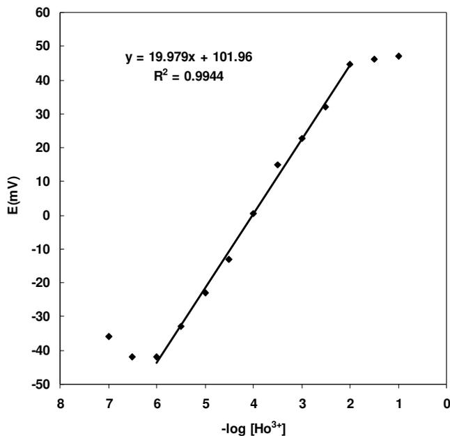
**Figure 2.** The calibration curve of the  $\text{Ho}^{3+}$  membrane sensor based on ATCD (membrane no. 4).
