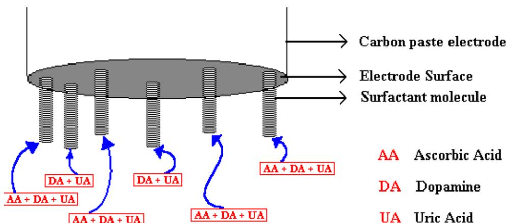
**Figure 7.** Schematic representation of carbon paste electrode comprising of surfactant molecules attached outside the electrode surface. AA, DA, and UA are getting attracted towards the surfactant modified carbon paste electrode which results in enhanced cyclic voltammograms responses.
