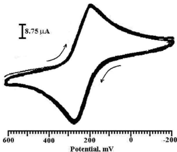
**Figure 1.** Cyclic voltammograms of  $\text{K}_3\text{Fe}(\text{CN})_6$  at Fe (II) ONTPc carbon paste electrode; supporting electrolyte,  $0.1 \text{ mol L}^{-1} \text{ KCl}$ ; scan rate  $100 \text{ mV s}^{-1}$ ; number of cycles are 20.
