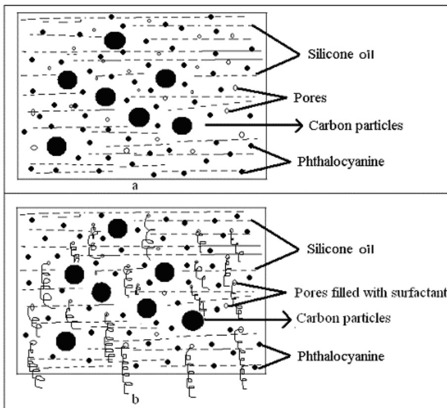
**Figure 6.** Schematic representation carbon paste electrode showing pores, carbon particles, phthalocyanine molecule and surfactant molecule on the surface of electrode.
