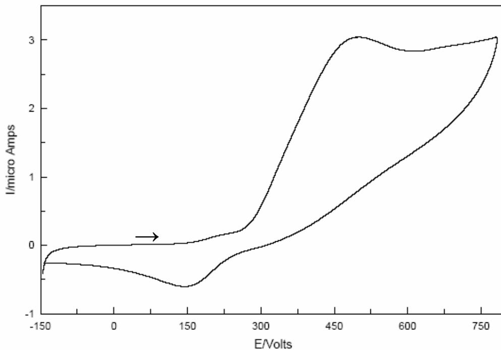
**Figure 4.** Cyclic voltammogram of 0.25 mM 3,4-dihydroxybenzaldehyde.
