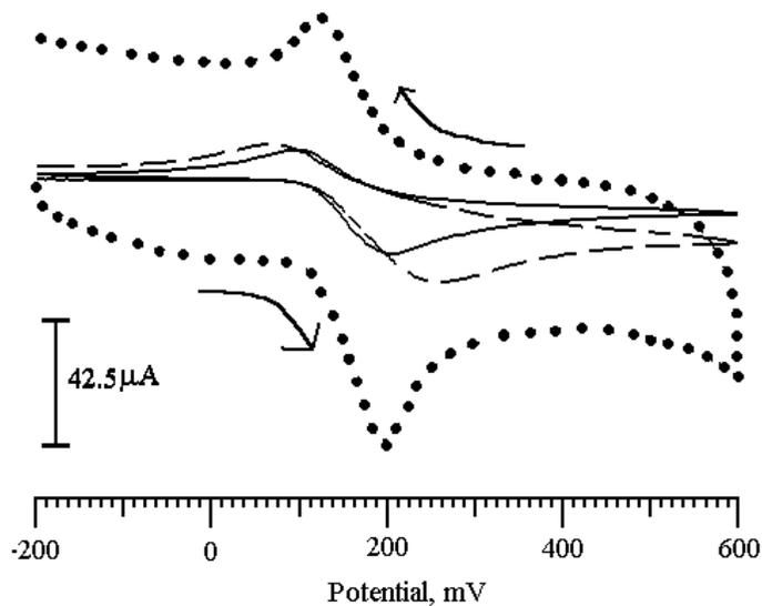
**Figure 7.** Cyclic voltammogram of DA for BCPE (solid line) LTGMCPE(line) and 35  $\mu\text{L}$  TX-100 dashed line
