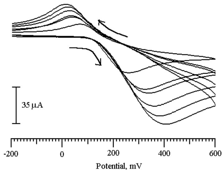
**Figure 5.** Cyclic voltammogram of DA at different concentration (  $0.1 \times 10^{-3}$  M,  $1.5 \times 10^{-3}$  M,  $2 \times 10^{-3}$  M,  $2.5 \times 10^{-3}$  M,  $3 \times 10^{-3}$  M,  $3.5 \times 10^{-3}$  M, ).
