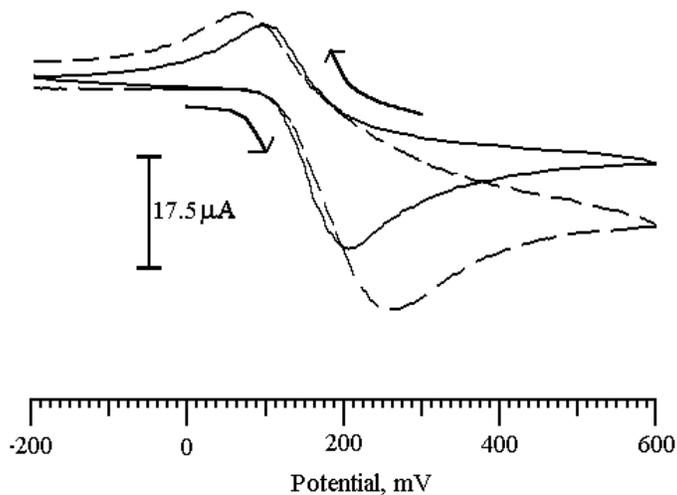
**Figure 2.** Cyclic voltammogram of  $1 \times 10^{-3}$  M DA in 0.2 M phosphate buffer solution of pH 7.0 at bare CPE (solid line) and LTGMCPPE (dashed line).
