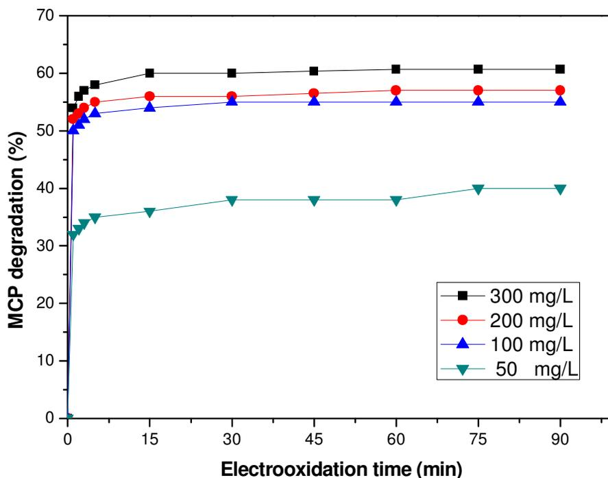
**Figure 3.** Percentage of MCP degradation by direct electrooxidation using titanium electrodes at a current density of  $50 \text{ A/m}^2$ .
