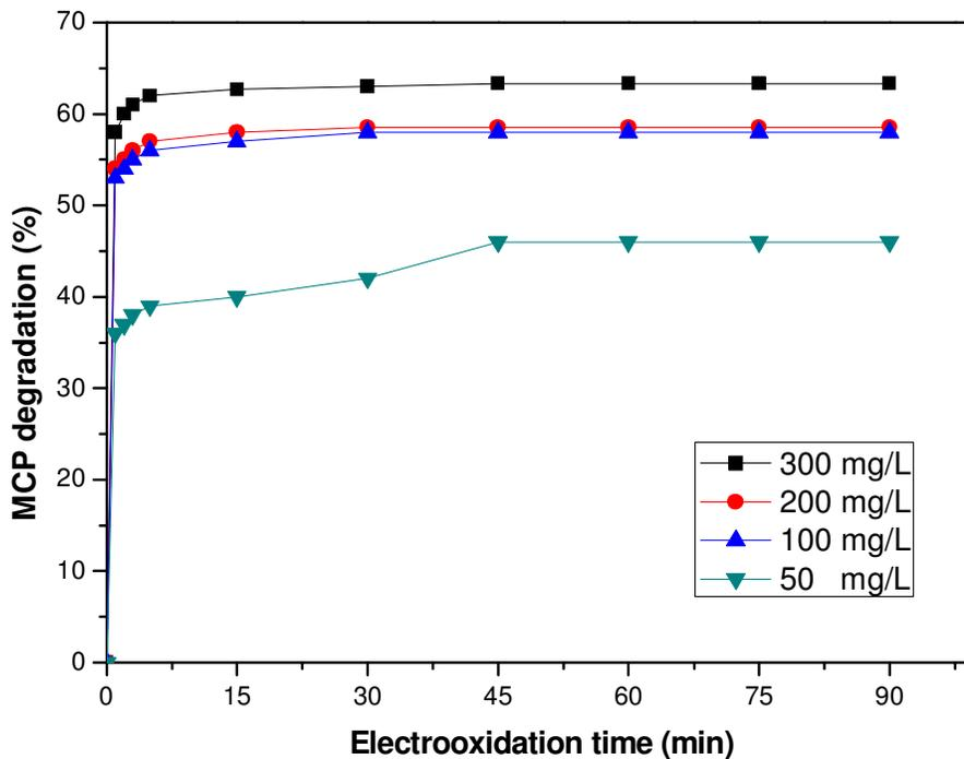
**Figure 4.** Percentage of MCP degradation by direct electrooxidation using titanium electrodes at a current density of 100 A/m<sup>2</sup>.
