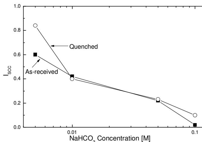
**Figure 4.** Effect of the NaHCO<sub>3</sub> concentration on the I<sub>SCC</sub> index value for the X-70 steel in the as-received and the quenched condition.
