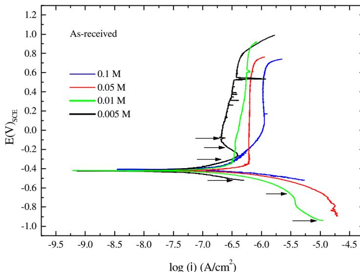
**Figure 2.** Effect of the  $\text{NaHCO}_3$  concentration on the polarization curves for the as-received X-70 steel. Arrows indicate the potentials, close to  $E_{\text{corr}}$ , at which SSRT tests were performed.
