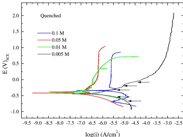
**Figure 3.** Effect of the NaHCO<sub>3</sub> concentration on the polarization curves for the quenched X-70 steel. Arrows indicate the potentials, closest to E<sub>corr</sub> at which SSRT tests were performed.
