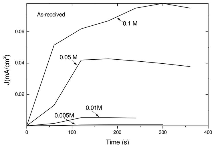
**Figure 9.** Effect of the  $\text{NaHCO}_3$  solution concentration on the hydrogen permeation current density for X-70 pipeline steel in the as-received condition.
