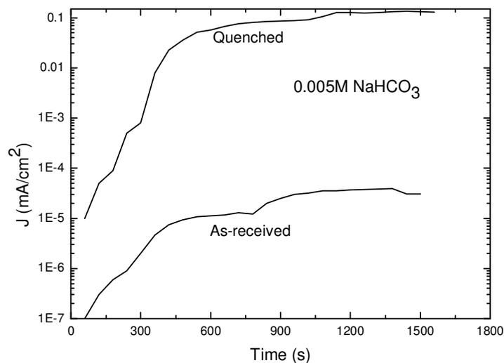
**Figure 10.** Effect of heat treatment on hydrogen permeation current density for X-70 pipeline steel in 0.005 M  $\text{NaHCO}_3$  solution.
