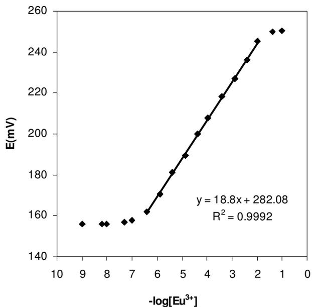
**Figure 2.** The calibration curve of the Eu(III) membrane sensor based on PMP
