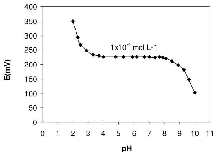
**Figure 3.** pH effect of the test solution on the potential response of the Eu(III) sensor
