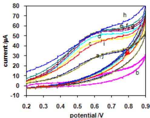
**Figure 9.** Laser reactivated cyclic voltammograms by  $N_2$  laser for oxidation process of  $5.00 \times 10^{-4} M$  cefazolin in the  $0.1 M Na_2CO_3$  solution (PH=11.7) at the glassy carbon electrode and scan rate  $50.0 mVs^{-1}$ . (Laser irradiation was non-simultaneous with electrochemical determination)
