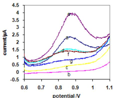
**Figure 12.** Laser reactivated differential pulse voltammograms by  $N_2$  laser for oxidation process of  $5.00 \times 10^{-4} M$  cefazolin in the  $0.1 M Na_2CO_3$  solution (PH=9.2) at the gold electrode and scan rate  $10.0 mVs^{-1}$ . (Laser irradiation was non-simultaneous with electrochemical determination)
