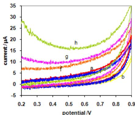
**Figure 3.** Electrochemical reactivated cyclic voltammograms for supporting electrolyte 0.1M Na<sub>2</sub>CO<sub>3</sub> solution (PH=11.7) at the glassy carbon electrode and scan rate 50.0mVs<sup>-1</sup>
