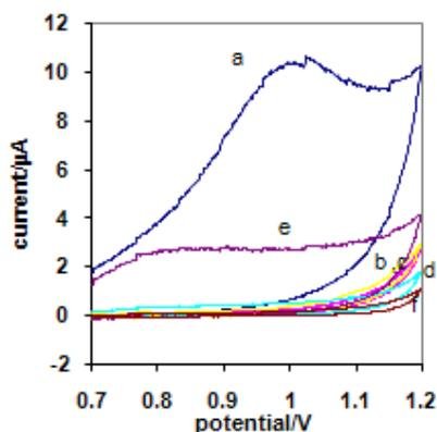
**Figure 6.** Anodic electrochemical reactivated Cyclic voltammograms for oxidation process of  $5.00 \times 10^{-4}$  M cefazolin in the 0.1M  $\text{Na}_2\text{CO}_3$  solution (PH=9.2) at the gold electrode and scan rate  $50.0 \text{ mVs}^{-1}$ .
