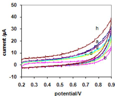
**Figure 10.** Laser reactivated cyclic voltammograms by  $N_2$  laser for supporting electrolyte  $0.1 M Na_2CO_3$  solution (PH=11.7) at the glassy carbon and scan rate  $50.0 mVs^{-1}$ . (Laser irradiation was non-simultaneous with electrochemical determination)
