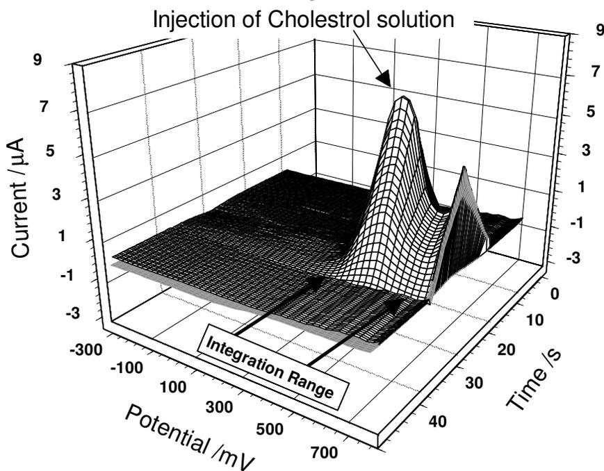
**Figure 3.** FFT cyclic voltammograms of the ChoX/ $\text{MnO}_2\text{NPs}/\text{MWNT}$ -modified GC electrode without (in absent) and with injection of  $200 \mu\text{L}$  of  $2.0 \times 10^{-5} \text{ M}$  cholesterol in  $0.01 \text{ M}$  PB at  $\text{pH}=7.4$  in the potential range of -200 to 700 mV at  $5 \text{ V/s}$ . and the potential Integration range for the current.
