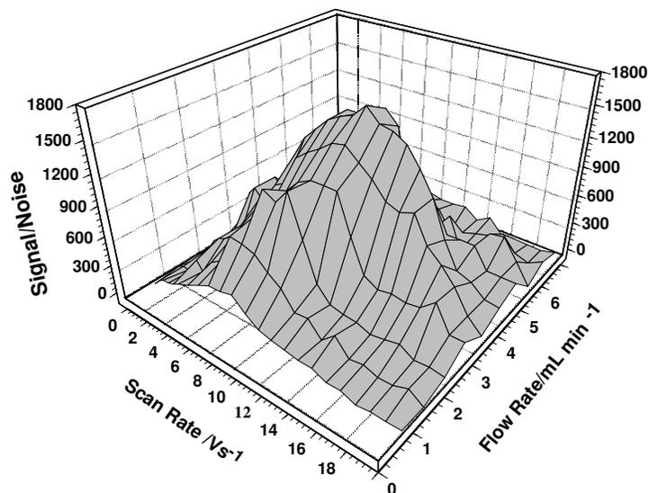
**Figure 4.** Effect of the sweep rate and effect of flow rate on the response of the ChoX/MnO<sub>2</sub>NPs/MWNT-modified GC electrode to injections of  $2.0 \times 10^{-5}$  M cholesterol
