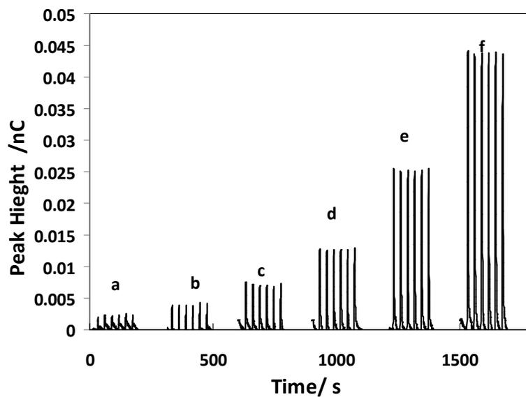
**Figure 5.** Response of the ChoX/MnO<sub>2</sub>NPs/MWNT-modified GC electrode to cholesterol in upon the following concentrations: a, 1; b, 2; c, 4; d, 8; e, 15; f, 25 nM.
