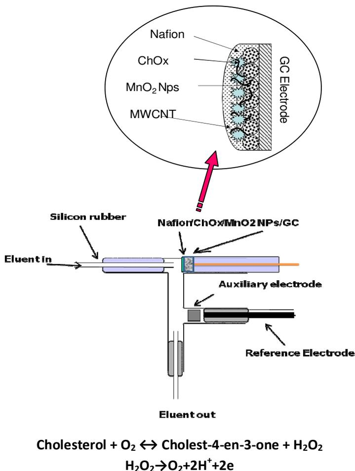
**Figure 2.** The diagram of cholesterol biosensor and the electrochemical cell used in flow injection analysis
