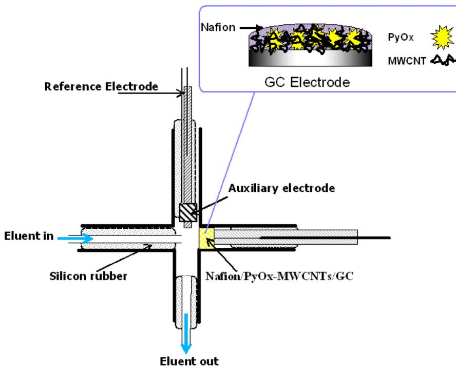
**Figure 2.** The diagram of phosphate ions biosensor and the electrochemical cell used in flow injection analysis
