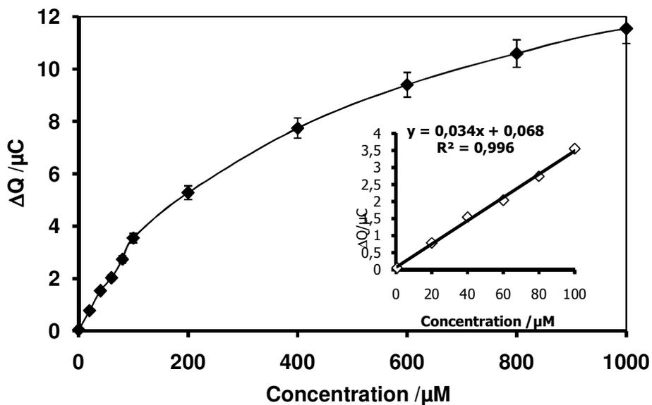
Figure 7. The calibration curve for phosphate ions determination
