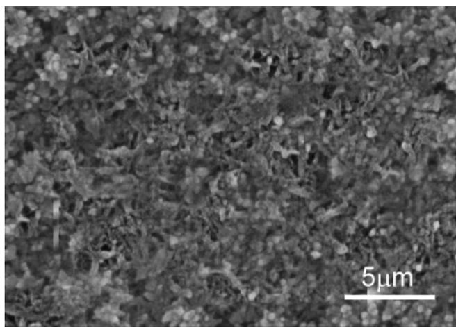
**Figure 3.** SEM image of the electrode PyOx-MWCNT/GC
