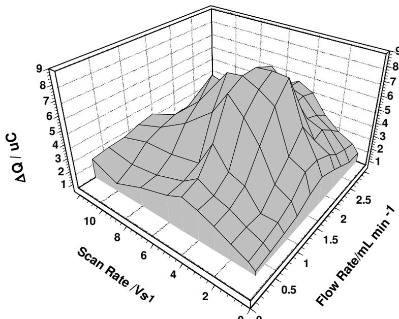
**Figure 6.** Effect of the sweep rate and effect of flow rate on the response of the Nafion/PyOx-MWCNTs modified GC electrode to injections of  $1.0 \times 10^{-4}$  M phosphate ions
