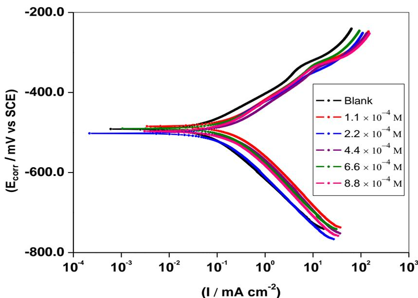
**Figure 7.** Tafel Polarization behavior of mild steel in 1 M HCl with different concentrations of Cefixime.
