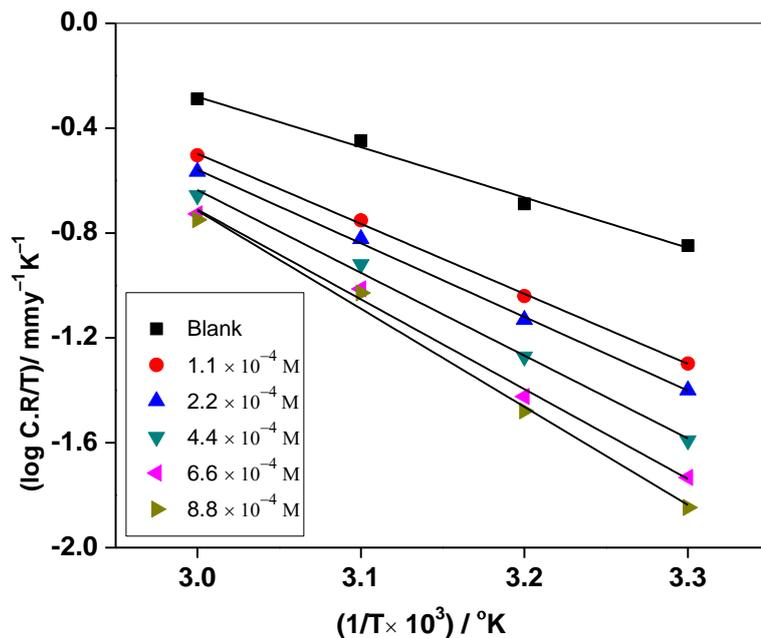
Figure 5. Adsorption isotherm plot for log (CR/T) vs. 1/T
