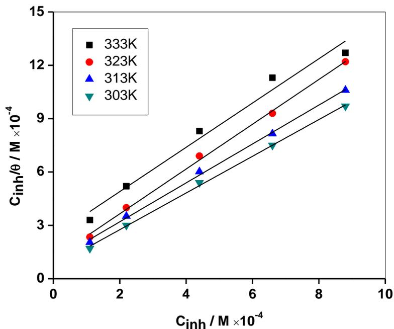
**Figure 3.** Langmuir's adsorption isotherm plots for the adsorption of Cefixime at different conc. in 1 M HCl on mild steel surface.
