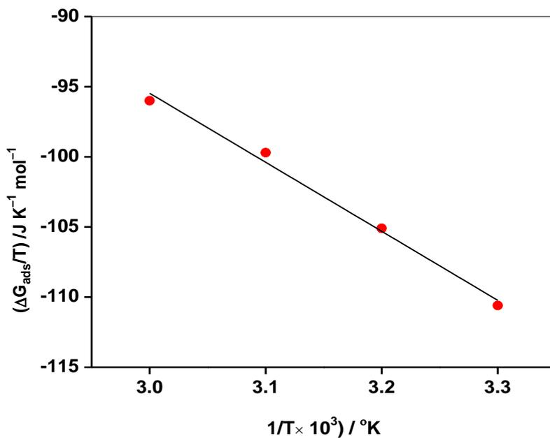
Figure 6. Adsorption isotherm plot for  $\Delta G_{ads}/T$  vs. 1/T.
