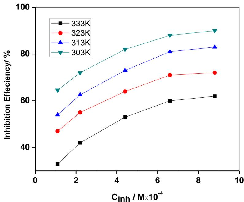
**Figure 2.** Variation of inhibition efficiency in 1 M HCl on mild steel with different conc. of Cefixime at different temperatures
