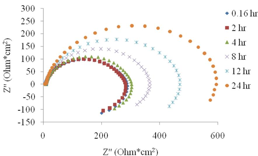
**Figure 14.** Effect of time on Nyquist plots of carbon steel in 4.0 M MEA /1.0[bmim] [DCA] at 40 °C and CO<sub>2</sub> loading of 0.55 mol/mol.
