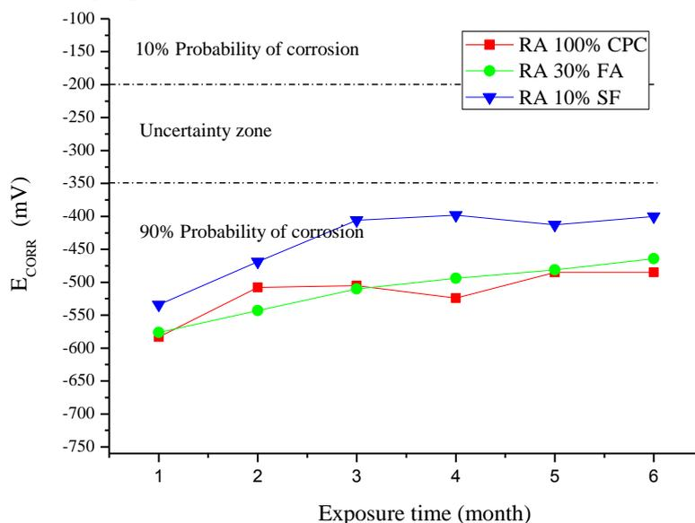
**Figure 3.** Variation of  $E_{\text{corr}}$  of the reinforcement steel as a function of the exposure time.
