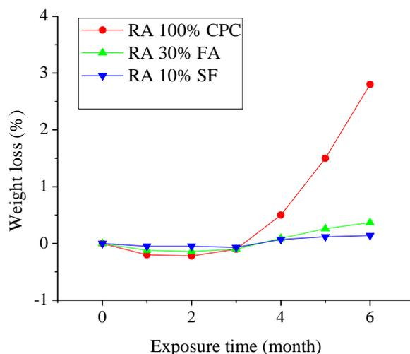
**Figure 2.** Weight loss of concrete in sulfate environment.
