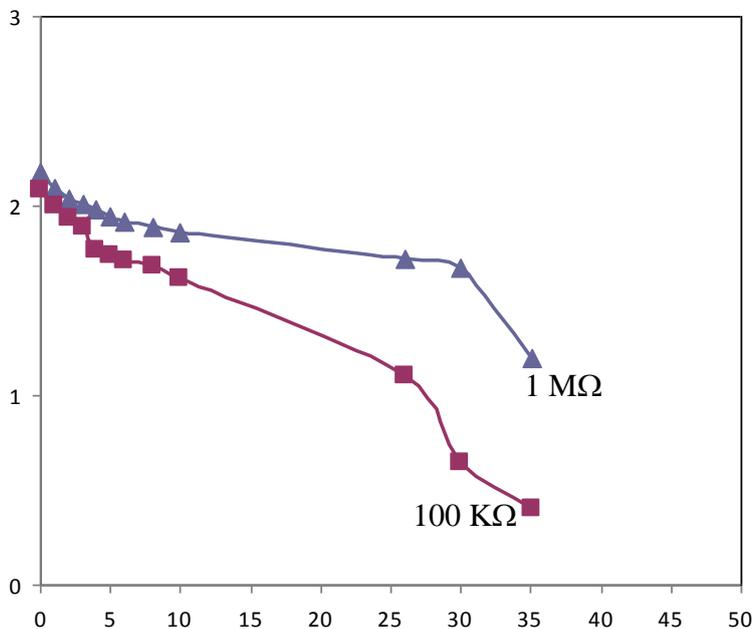
Figure 13. Cell potential discharge profile as a function of time for Cell # 1: (▲) 1 MΩ, (■) 100 K Ω.
