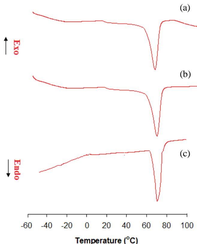
**Figure 12.** DSC thermograms for: (a) pure PEO, (b) SPE host: (70PEO:30KNO<sub>3</sub>), (c) (70PEO:30KNO<sub>3</sub>) + 5 % SiO<sub>2</sub>
