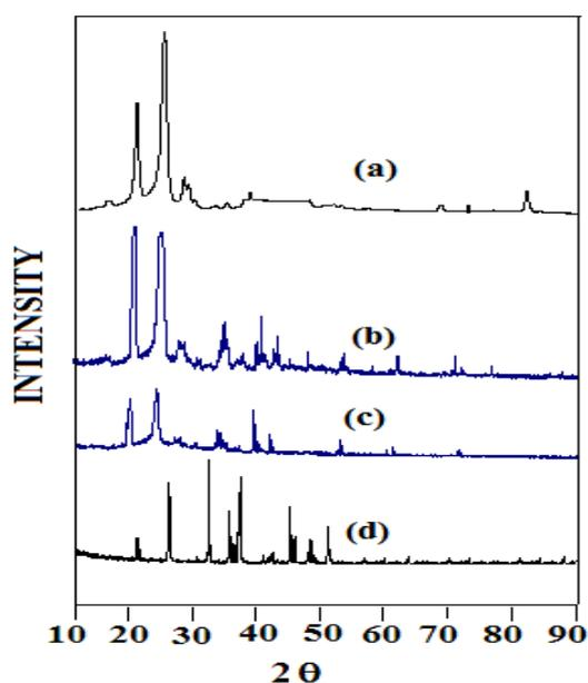
**Figure 10.** XRD pattern for (a) Pure PEO, (b) SPE host: (70PEO: 30KNO<sub>3</sub>), (c) NCPE: (70PEO: 30 KNO<sub>3</sub>) + 5SiO<sub>2</sub>, (d) KNO<sub>3</sub>.
