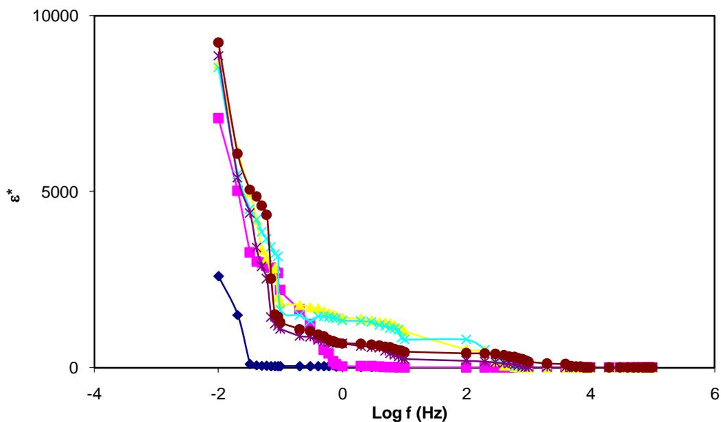
Figure 8. The frequency response of complex dielectric constant ( $\epsilon^*$ ) for NCPE film at different temperatures: ( $\blacklozenge$ ) 303, ( $\blacksquare$ ) 313, ( $\Delta$ ) 323, ( $+$ ) 333, ( $\circ$ ) 343, ( $-$ ) 353 <sup>0</sup>K.
