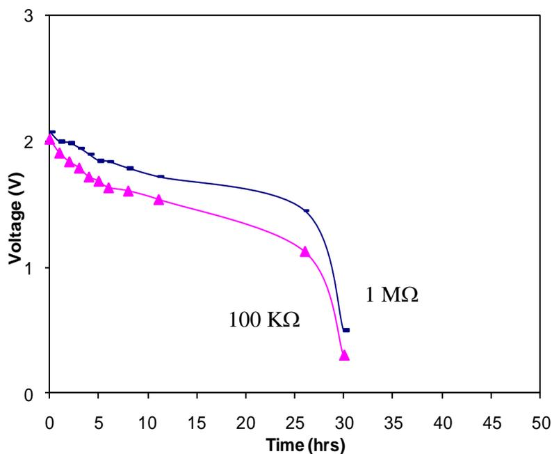
Figure 14. Cell potential discharge profile as a function of time Cell # 2: (▲) 100 KΩ, (-) 1 M Ω.
