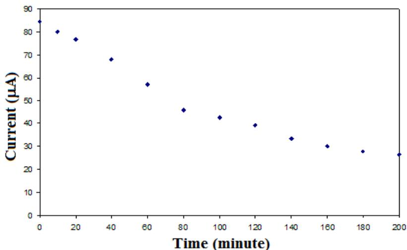
Figure 7. Polarization current versus time plot for the cell: K// NCPE film// K
