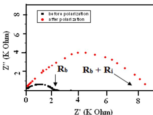
**Figure 6.** Complex impedance ( $Z'$ - $Z''$ ) plots before and after cell polarization
