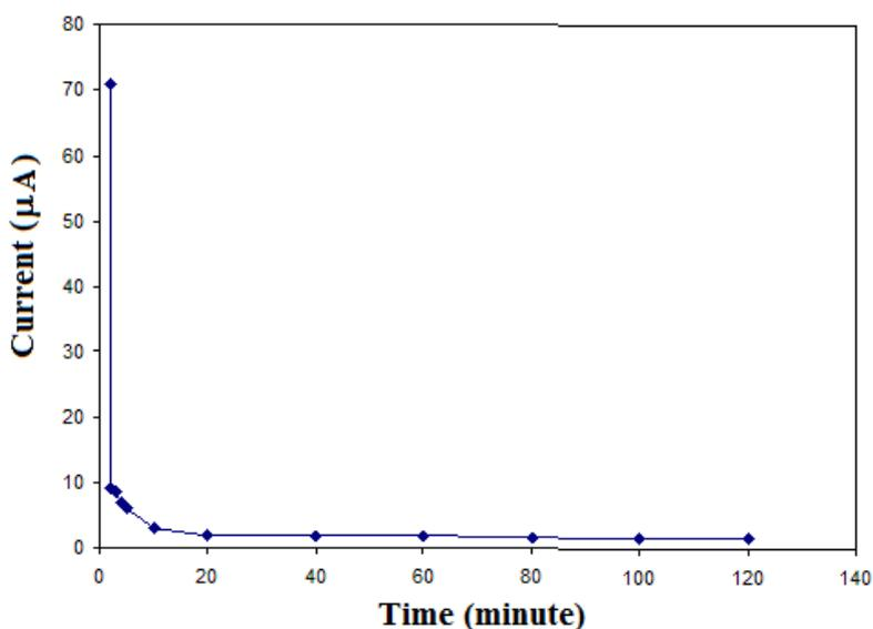
**Figure 5.** Variation of polarizing current as a function of time in a typical cell: SS//NCPE film// SS
