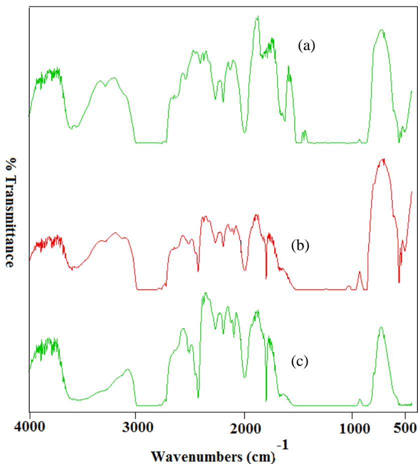
**Figure 11.** FTIR spectrographs for (a) Pure PEO, (b) SPE host: (70PEO:30KNO<sub>3</sub>), (c) NCPE: (70PEO: 30KNO<sub>3</sub>) + 5 % SiO<sub>2</sub>.
