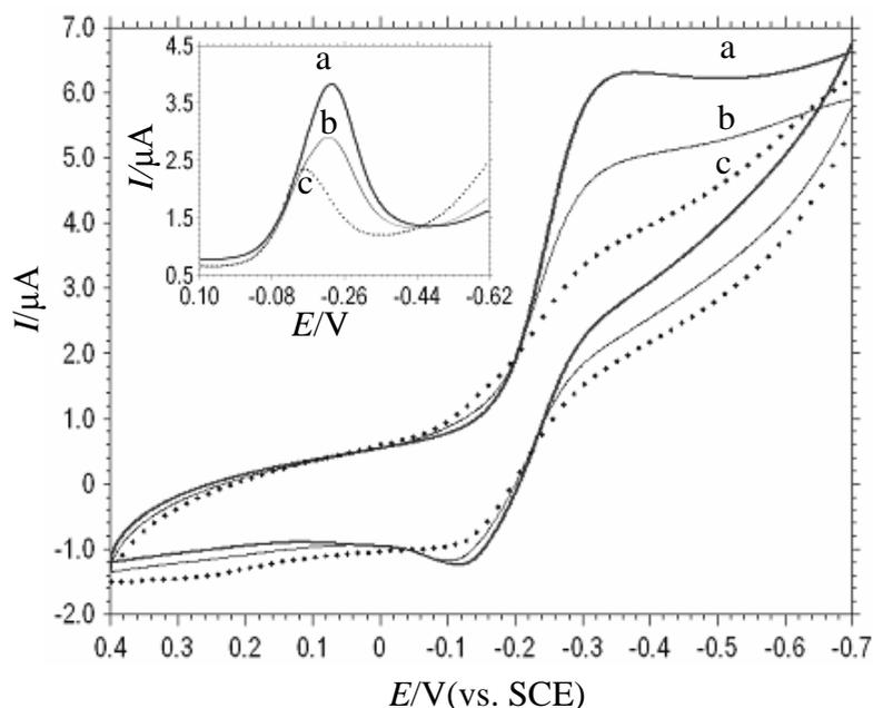
**Figure 1.** CVs (main panel) and DPVs (inset) of 300  $\mu\text{M}$   $[\text{Cu}(\text{bpy})(\text{MBZ})_2(\text{H}_2\text{O})]$  in the absence (a) and in the presence of 33  $\mu\text{M}$  dsDNA (b) or ssDNA (c) in 20 mM pH 7.1 Tris-HCl. Scan rate for CV: 40  $\text{mV s}^{-1}$ . DPV conditions: amplitude, 0.05 V; pulse width, 0.05 s; pulse width, 0.2 s.
