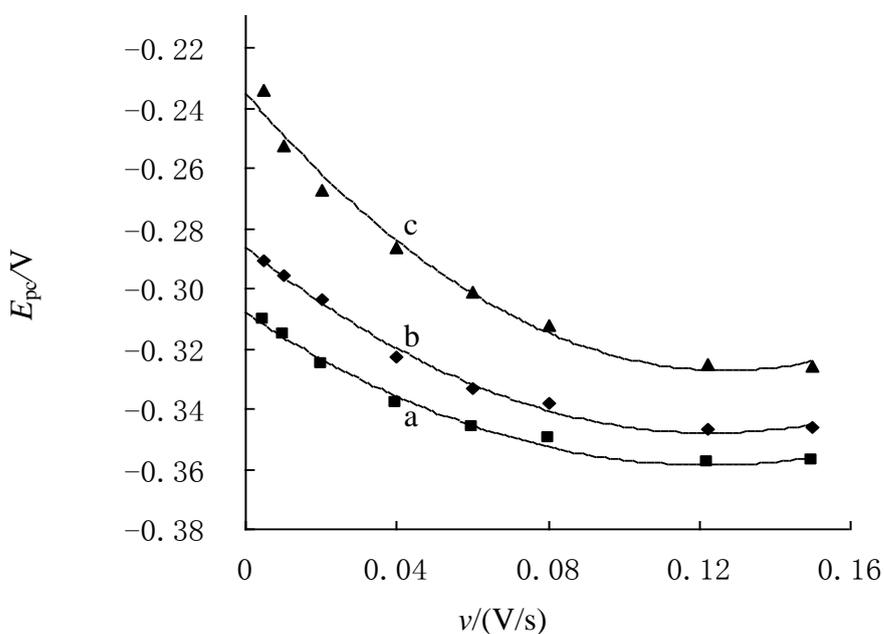
**Figure 3.** Relationships between reduction peak potentials ( $E_{pc}$ ) and scan rate ( $v$ ) of 300  $\mu\text{M}$   $[\text{Cu}(\text{bpy})(\text{MBZ})_2(\text{H}_2\text{O})]$  in the absence (a) or presence of 33  $\mu\text{M}$  dsDNA (b) and ssDNA (c). Supporting electrolyte was 20 mM pH 7.1 Tris-HCl
