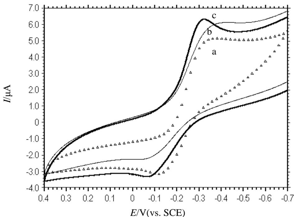
**Figure 5.** CVs of 300  $\mu\text{M}$  [Cu(bpy)(MBZ)<sub>2</sub>(H<sub>2</sub>O)] in 20 mM pH 7.1 Tris-HCl buffer at bare GCE (a), ssDNA/GCE (b) and dsDNA/GCE (c). Scan rate = 40  $\text{mV s}^{-1}$ .
