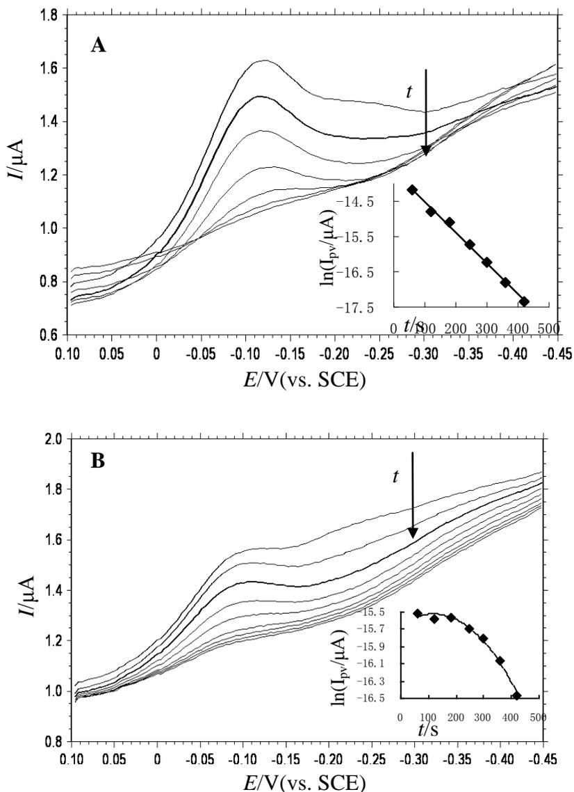
**Figure 6.** Time-dependent DPVs obtained in 20 mM pH 7.1 Tris-HCl at dsDNA/GCE (A) and ssDNA/GCE (B) after immersing the modified electrodes into 300  $\mu\text{M}$   $[\text{Cu}(\text{bpy})(\text{MBZ})_2(\text{H}_2\text{O})]$  for equilibrium. Insets: plots of  $\ln I_{\text{pc}}$  versus dissociation time ( $t$ ) obtained from dsDNA/GCE (A) and ssDNA/GCE (B)
