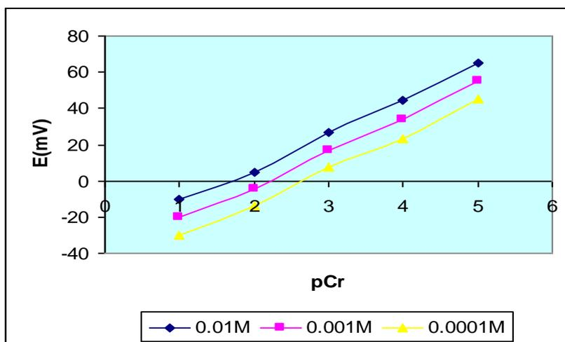
**Figure 3.** Effect of internal solution on the response of electrode.
