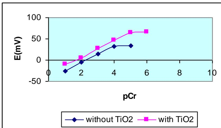
**Figure 2.** Calibration plot of the Cr(III)-ISE based on ligand.
