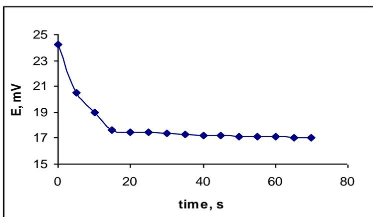
Fig. 3. The response time of Cr(III)-ISE based on ligand for Cr(III) concentration of 1.0 × 10<sup>-4</sup> M.
