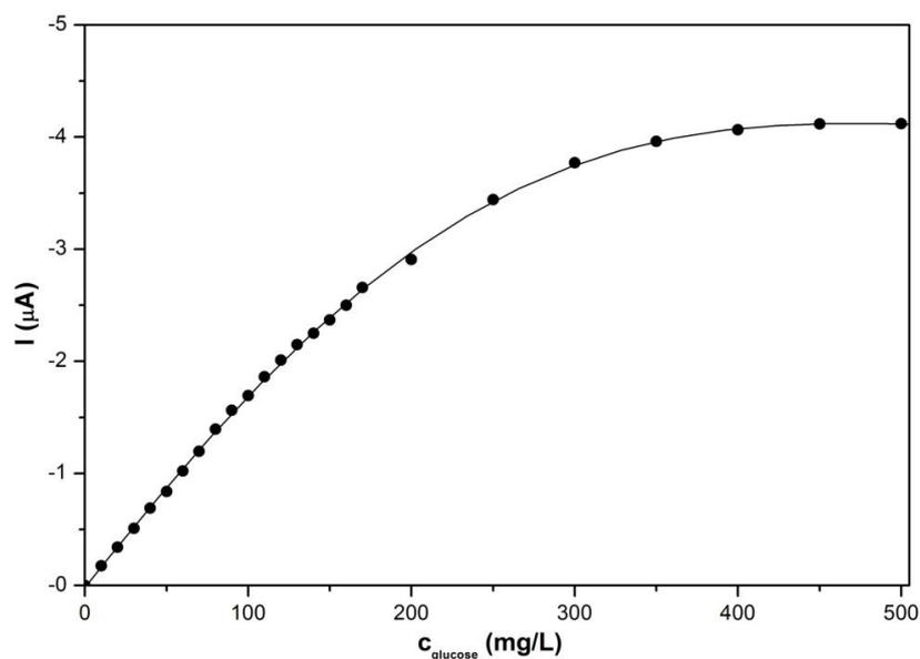
**Figure 6.** Relation between current response and glucose concentration. Experimental conditions:  $c(\text{GLU}) = 1\text{-}500$  ppm;  $E_{\text{det}} = -400$  mV; phosphate buffer (pH 7.5). For other conditions, see Fig.2.
