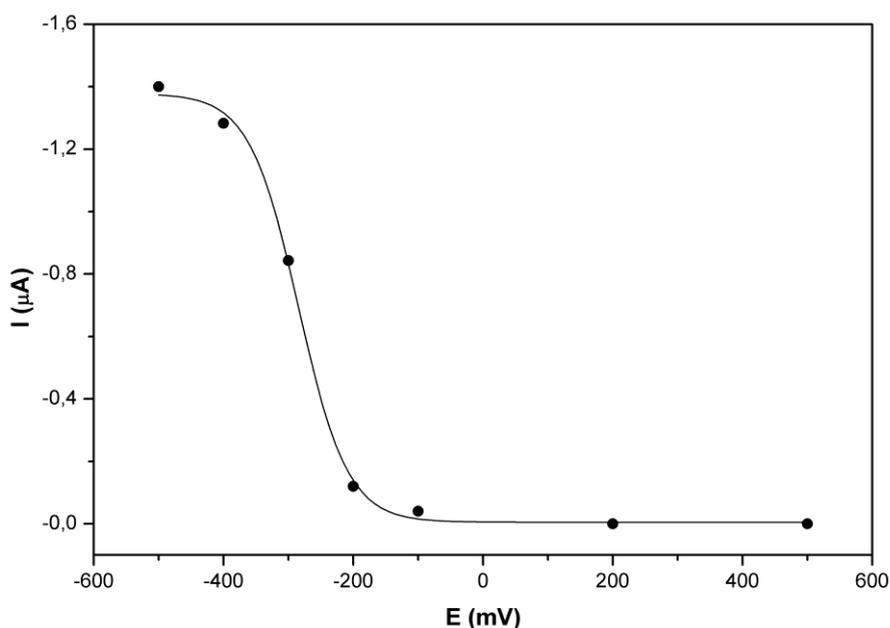
**Figure 4.** Effect of potential on the CPE/PANI/GOD sensor response. Experimental conditions:  $E^{\text{det}} = -500$  to  $+500$  mV. For other conditions, see Fig.2.
