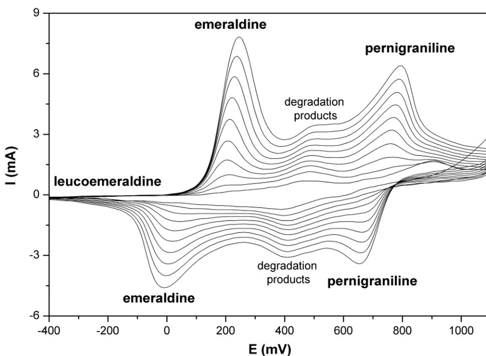
**Figure1.** Electrochemical synthesis of PANI. Experimental conditions: 0.2M aniline monomer in 1MHCl. Cyclic voltammetry; potential limits:  $E_{\text{low}} = -400$  mV;  $E_{\text{high}} = +1200$  mV, initial potential,  $E_{\text{init}} = +1200$  mV; scan rate,  $v = 100$   $\text{mV s}^{-1}$ ; number of cycles,  $n = 10$ .
