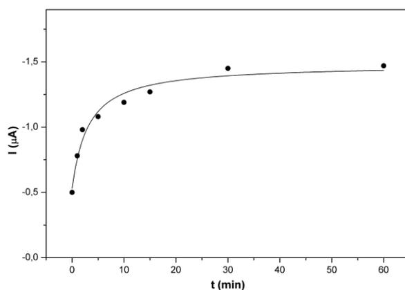
**Figure 3.** Effect of time on the GOD immobilization. Experimental conditions:  $E_{\text{imb}} = +700$  mV;  $t_{\text{imb}} = 0$ -60 min.  $E_{\text{det}} = -400$  mV. For other conditions, see Fig.2 and legend.
