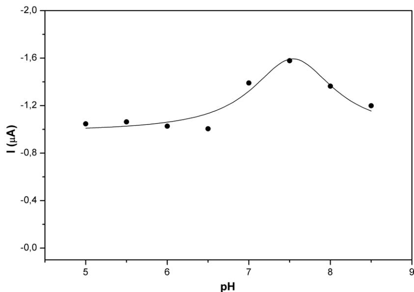
**Figure 5.** Effect of pH on the CPE / PANI / GOD sensor response. Experimental conditions:  $E_{\text{det}} = -400$  mV; a set of phosphate buffers (pH 5.0 – 8.5). For other conditions, see Fig.2.
