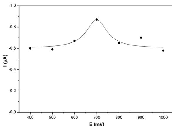
**Figure 2.** Effect of applied potential on the GOD immobilization. Experimental conditions: GOD immobilization conditions:  $E_{\text{imb}} = +400$  to  $+1000$  mV vs. ref.,  $t_{\text{imb}} = 30$  min;  $c(\text{GOD}) = 0.75$  mg mL<sup>-1</sup> in phosphate buffer (pH 7.5); Test solution: phosphate buffer (pH 7.5),  $c(\text{GLU}) = 100$  mg L<sup>-1</sup>; detection potential,  $E_{\text{det}} = -300$  mV.
