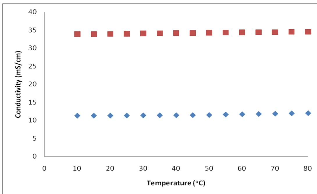
**Figure 7.** Plot of conductivity of ethanol (♦) pure 1-butyl-3-methylimidazolium bromide [BMIm][Br] in ethanol (■) as a function of temperature.
