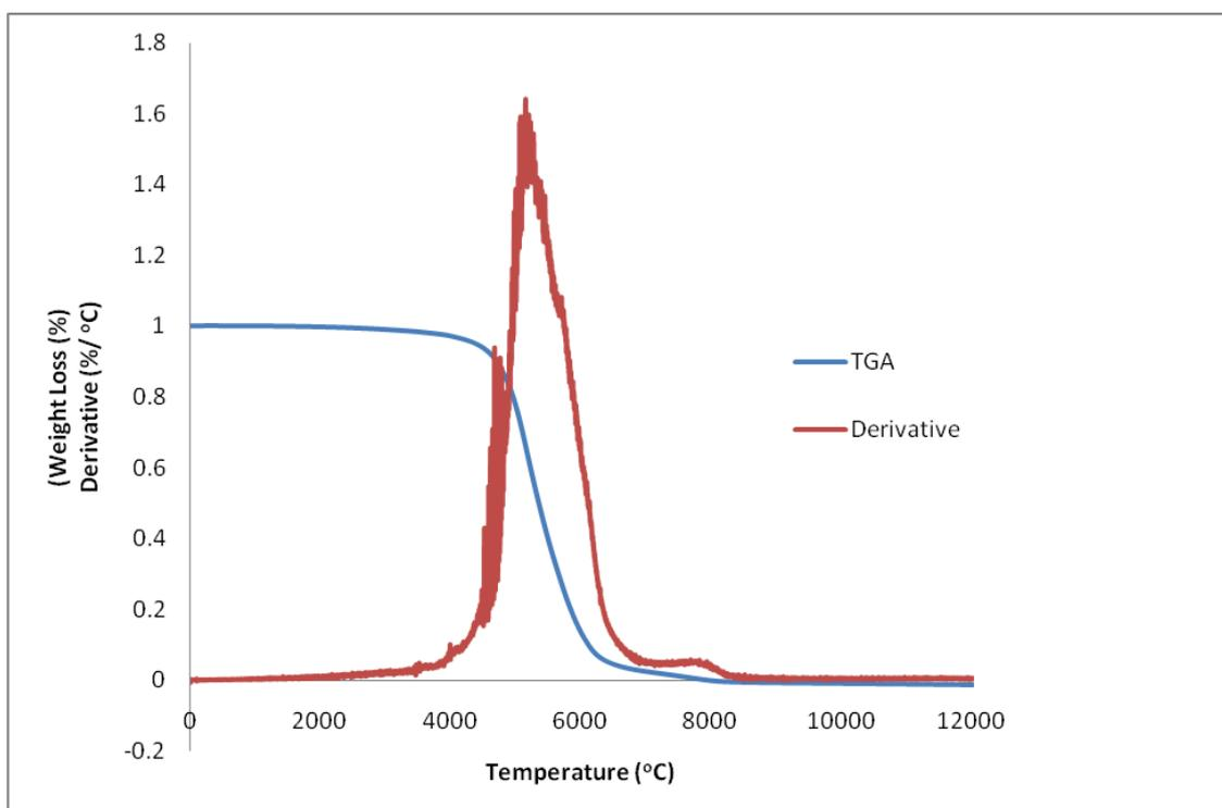
**Figure 11.** Thermogravimetric analysis (TGA) and derivative thermogravimetric analysis of [BMIm][Br].
