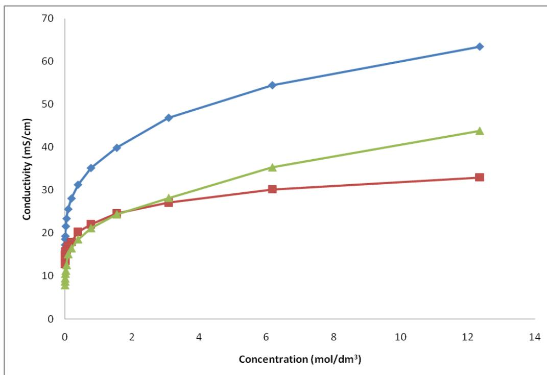
**Figure 10.** Plot of conductivity at different concentrations of [BMIm][Br] against the solvents water (♦), acetonitrile (■) and methanol (▲) at ambient temperature.
