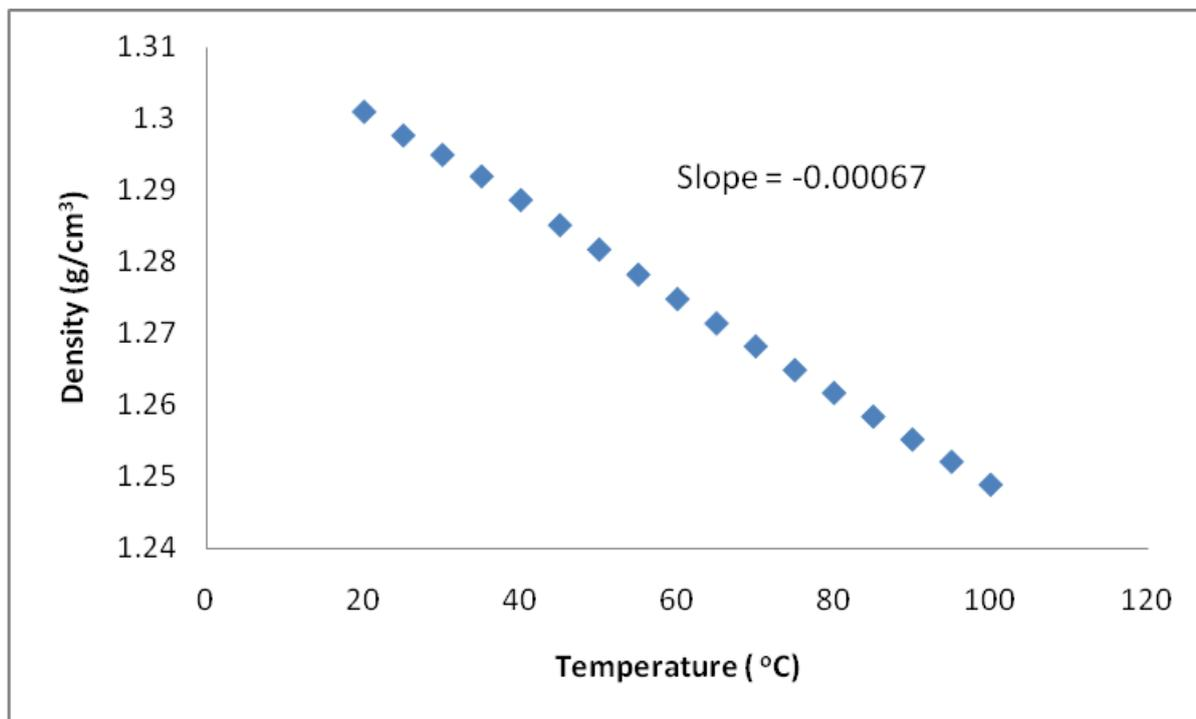
**Figure 1.** Density measurement of pure 1-butyl-3-methylimidazolium bromide [BMIm][Br] as a function of temperature.
