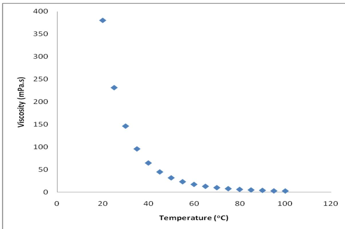
**Figure 2.** Viscosity measurement of pure 1-butyl-3-methylimidazolium bromide [BMIm][Br] as a function of temperature.
