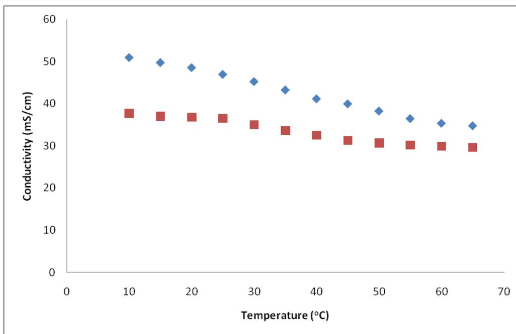
**Figure 6.** Plot of conductivity of methanol (♦) and pure 1-butyl-3-methylimidazolium bromide [BMIm][Br] in methanol (■) as a function of temperature.
