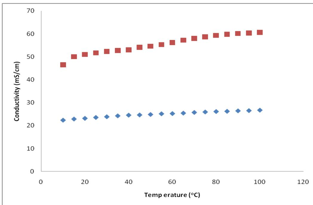
**Figure 5.** Plot of conductivity of water (◆) and pure 1-butyl-3-methylimidazolium bromide [BMIm][Br] in water (■) as a function of temperature.
