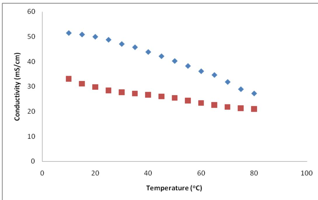
**Figure 8.** Plot of conductivity of acetonitrile (◆) pure 1-butyl-3-methylimidazolium bromide [BMIm][Br] in acetonitrile (■) as a function of temperature.
