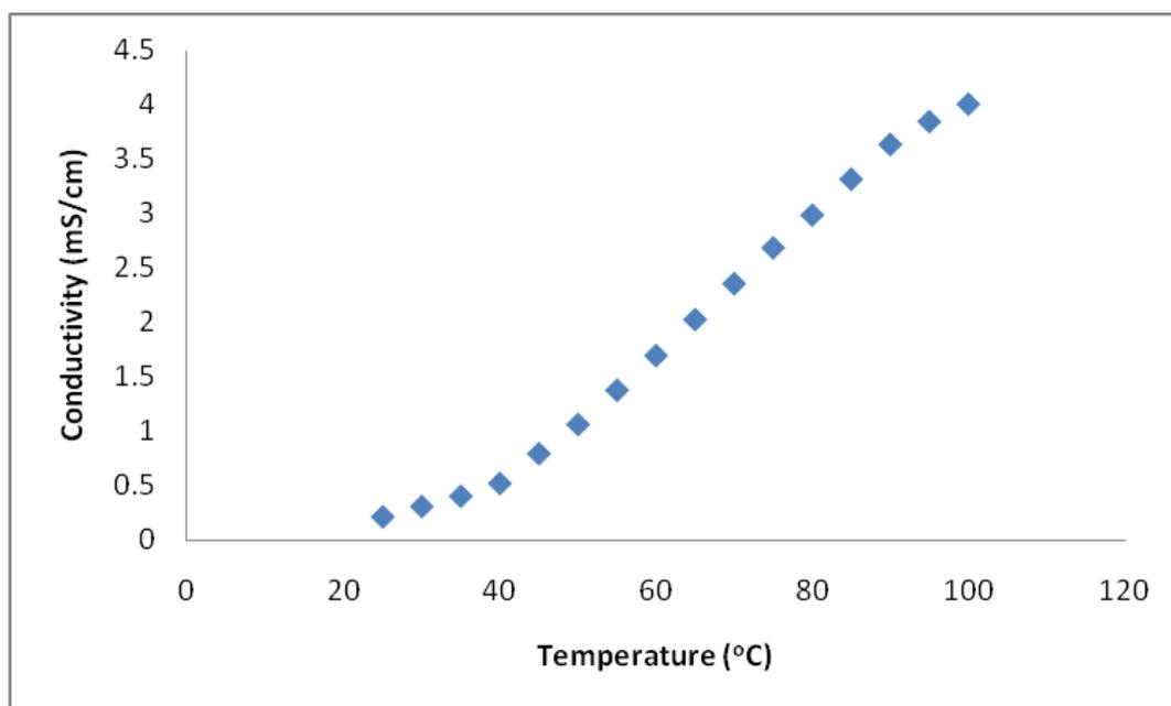
**Figure 4.** Plot of conductivity of pure 1-butyl-3-methylimidazolium bromide [BMIm][Br] as a function of temperature.
