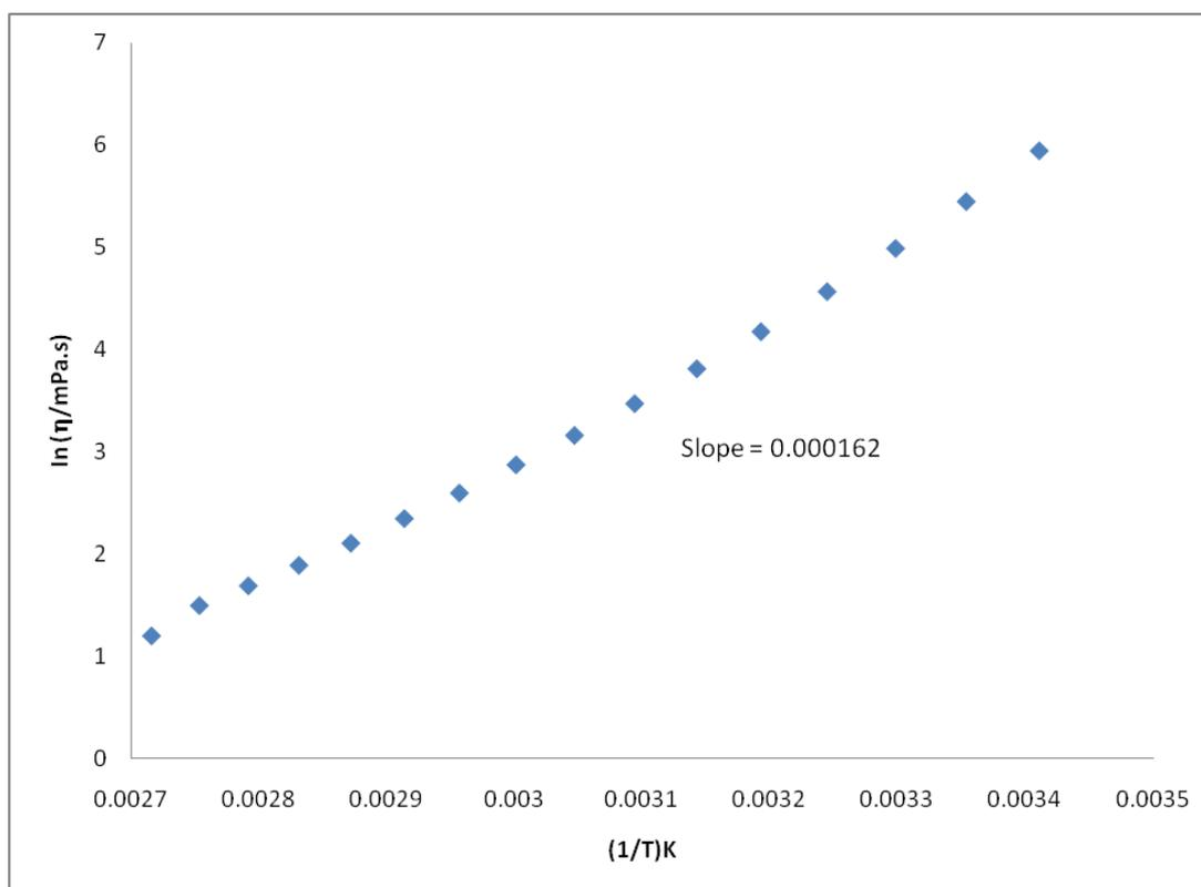
**Figure 3.** Arrhenius plot of viscosity of pure 1-butyl-3-methylimidazolium bromide [BMIm][Br] as a function of inverse of temperature.
