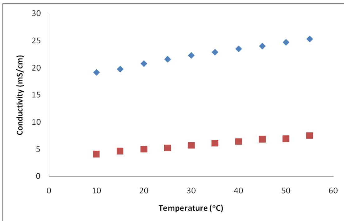
**Figure 9.** Plot of conductivity of acetone (◆) pure 1-butyl-3-methylimidazolium bromide [BMIm][Br] in acetone (■) as a function of temperature.
