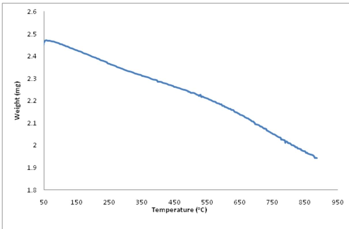
**Figure 6.** Thermogravimetric analysis graph of soot obtained from the atmospheric combustion of diesel fuel.
