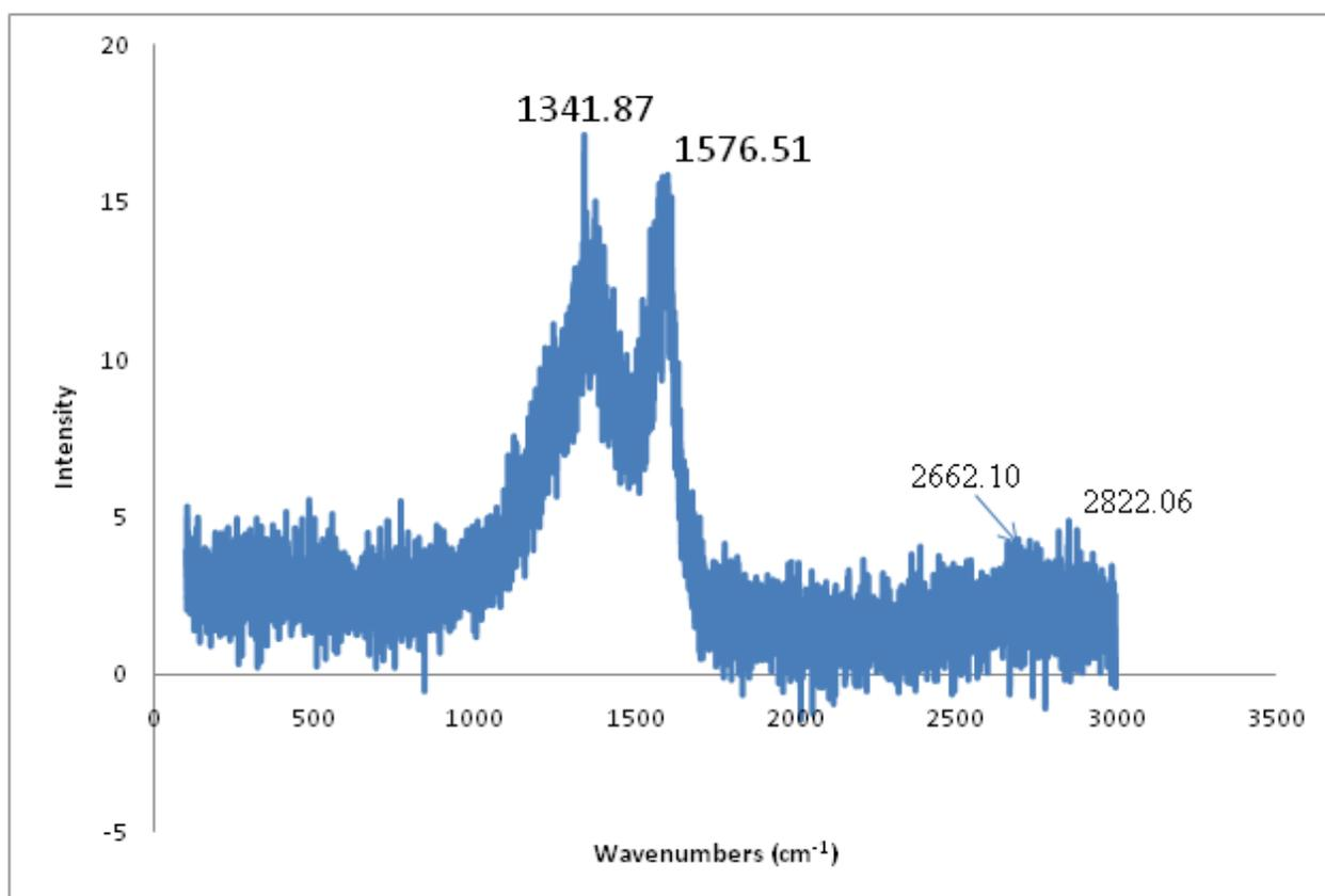
**Figure 3.** Raman spectra of soot obtained from the atmospheric combustion of diesel.
