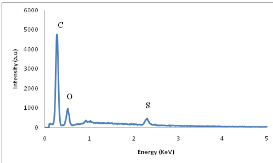
**Figure 2.** Energy dispersive spectroscopy (EDS) spectra of soot obtained from the atmospheric combustion of diesel.
