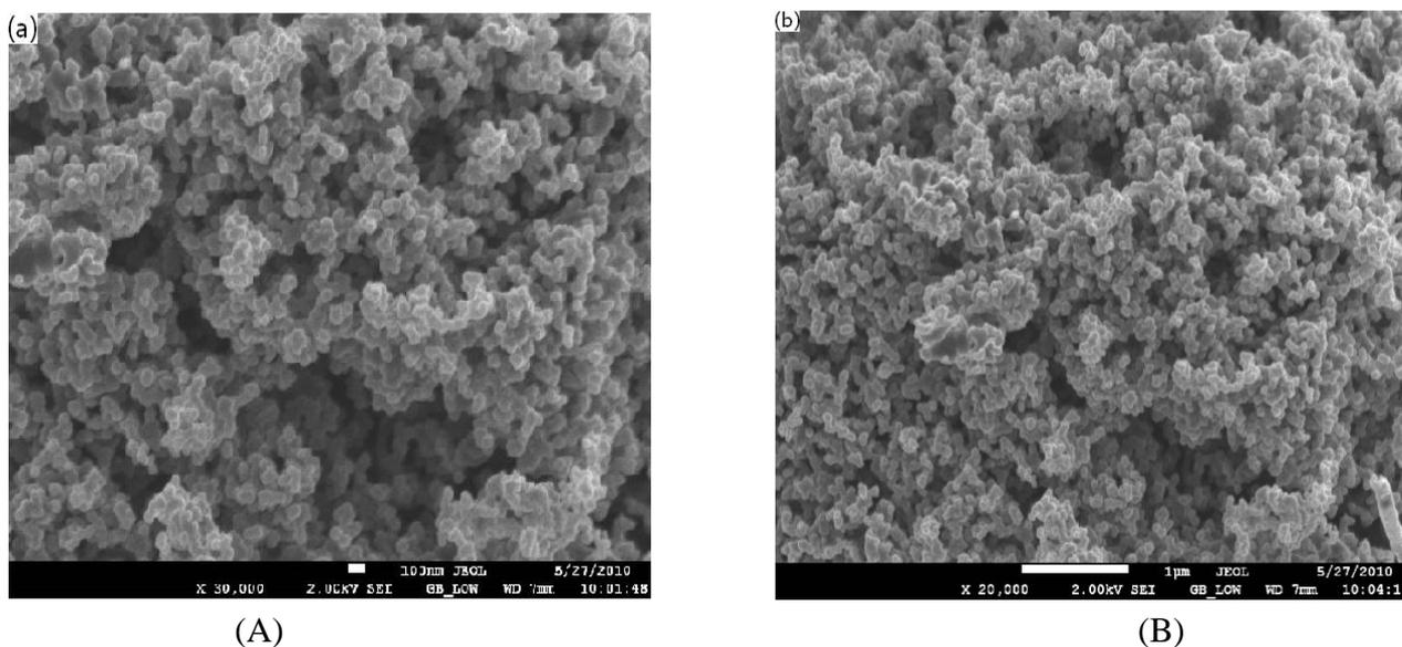
**Figure 1.** Scanning electron micrograph (FE-SEM) of soot obtained from the atmospheric combustion of diesel.
