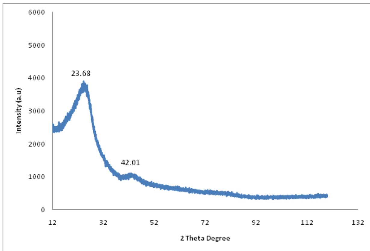
**Figure 4.** X-ray diffraction spectra of soot obtained from the atmospheric combustion of diesel.
