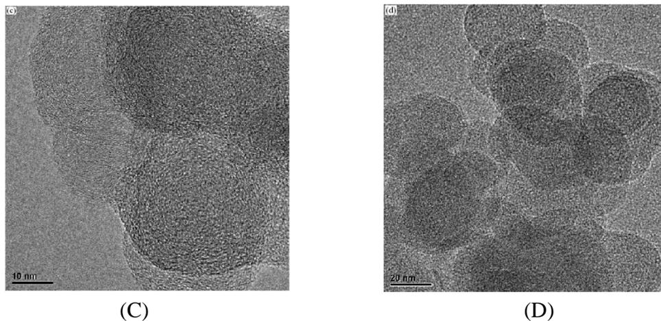
**Figure 5.** HR-TEM micrograph of soot obtained from the atmospheric combustion of diesel.
