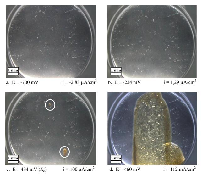
**Figure 2.** images of the Alloy 31 surface at different points of the polarization curve in the 700 g/l LiBr solution at 50°C
