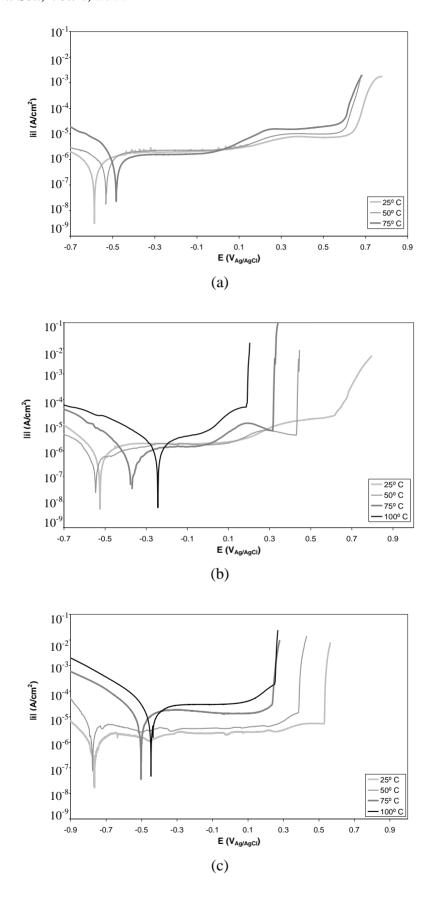
**Figure 1.** Potentiodynamic polarization curves for Alloy 31 at different temperatures for (a) 400 g/l LiBr, (b) 700 g/l LiBr and (c) 992 g/l LiBr solutions.
