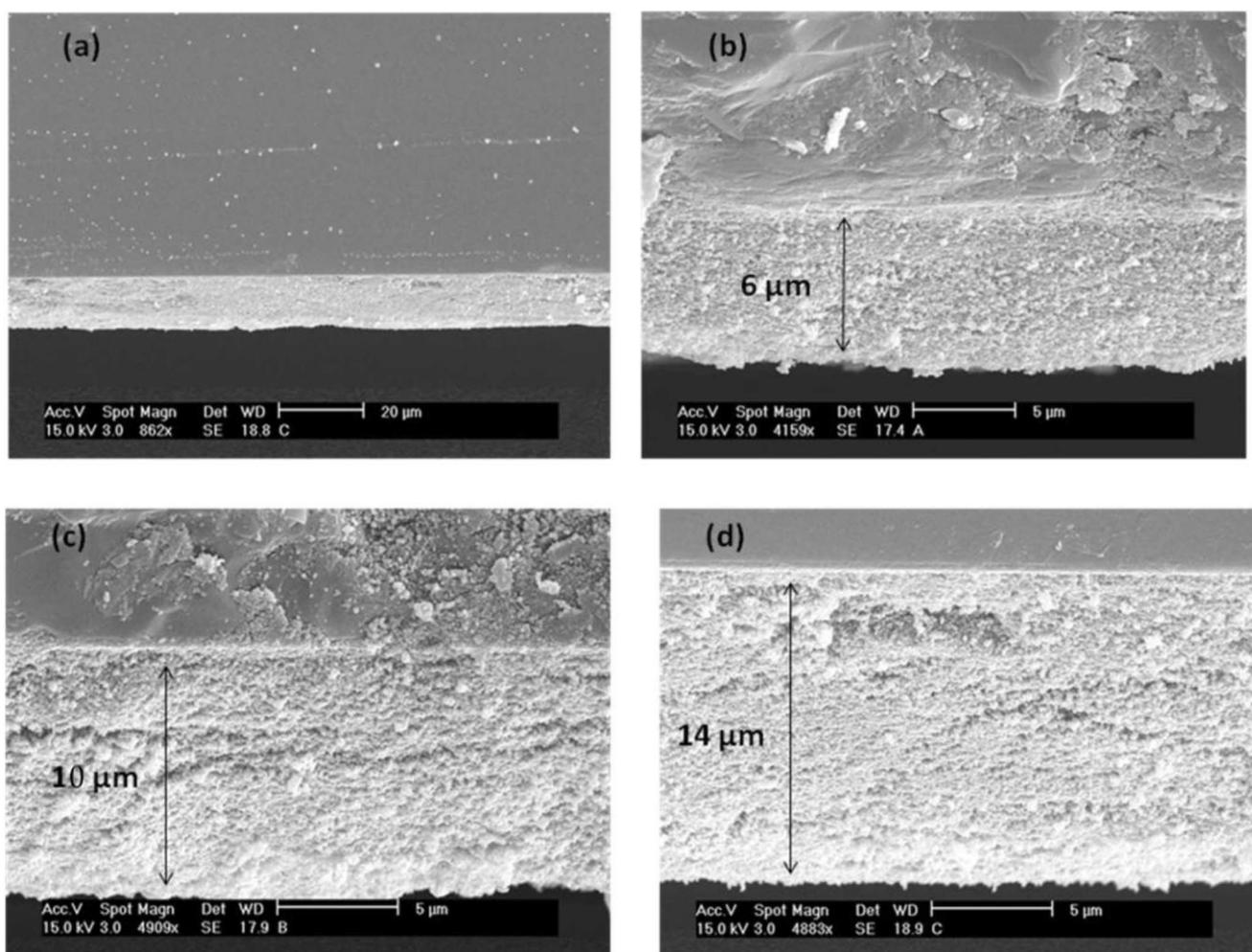
**Figure 1.** SEM cross-sectional images of  $\text{TiO}_2$ -coated FTO glasses at low magnification (a) and at high magnification (b), (c) and (d) with the estimation of  $\text{TiO}_2$  thickness.
