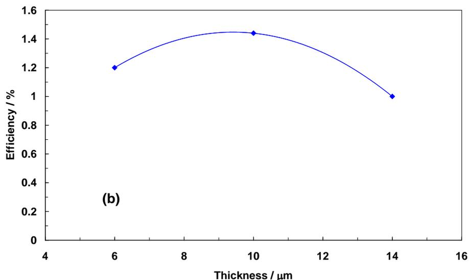
**Figure 5.** Variation of Fill Factor (a) and Efficiency (b) as a function of  $\text{TiO}_2$  thickness of the photoanodes.
