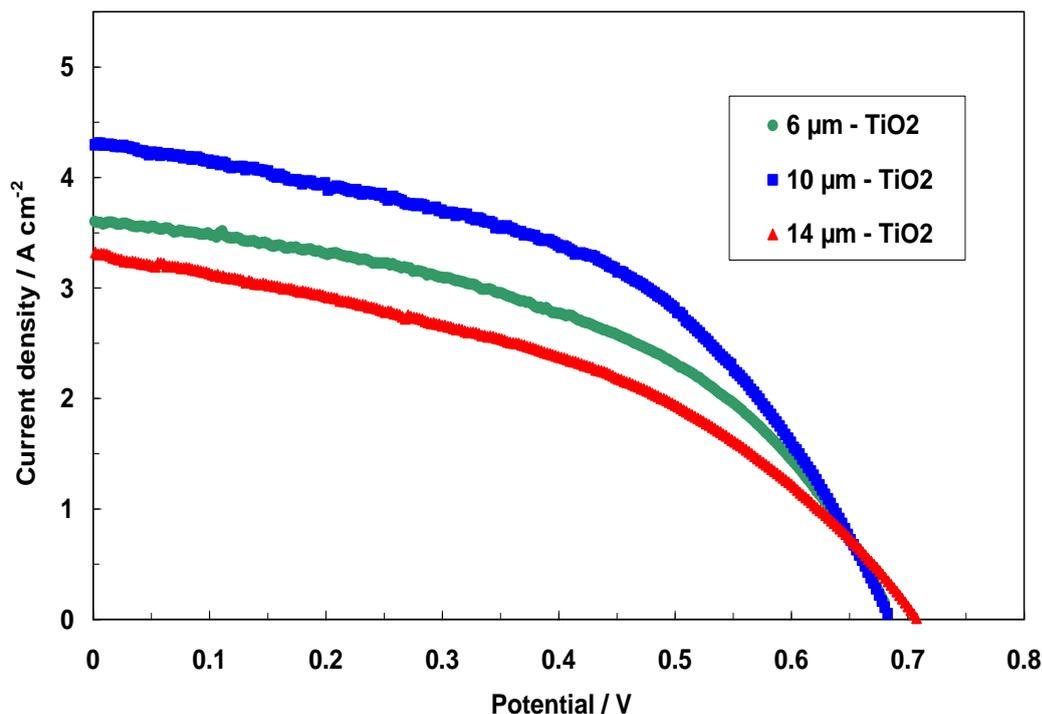
**Figure 2.** j–V curves for DSSCs using TiO<sub>2</sub> at different thicknesses as photo-anodes.
