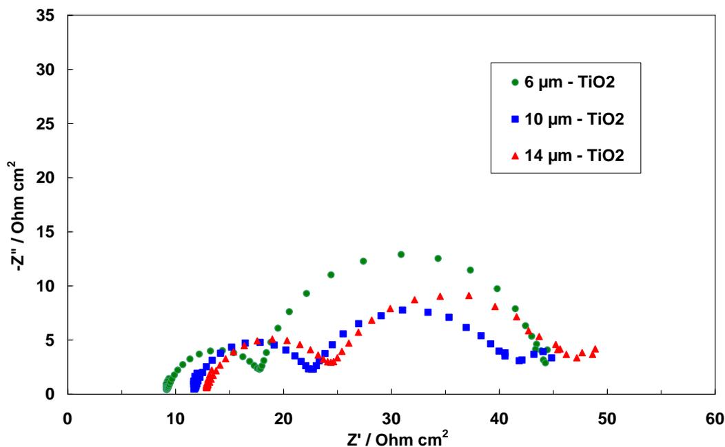
**Figure 6.** Electrochemical Impedance Spectra for DSSCs using  $\text{TiO}_2$  at different thicknesses as photoanodes.
