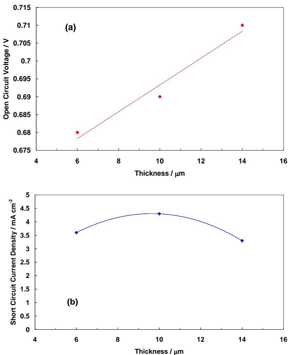
**Figure 3.** Variation of Open Circuit Voltage (a) and Short Circuit Current Density (b) as a function of TiO<sub>2</sub> thickness of the photo-anodes.
