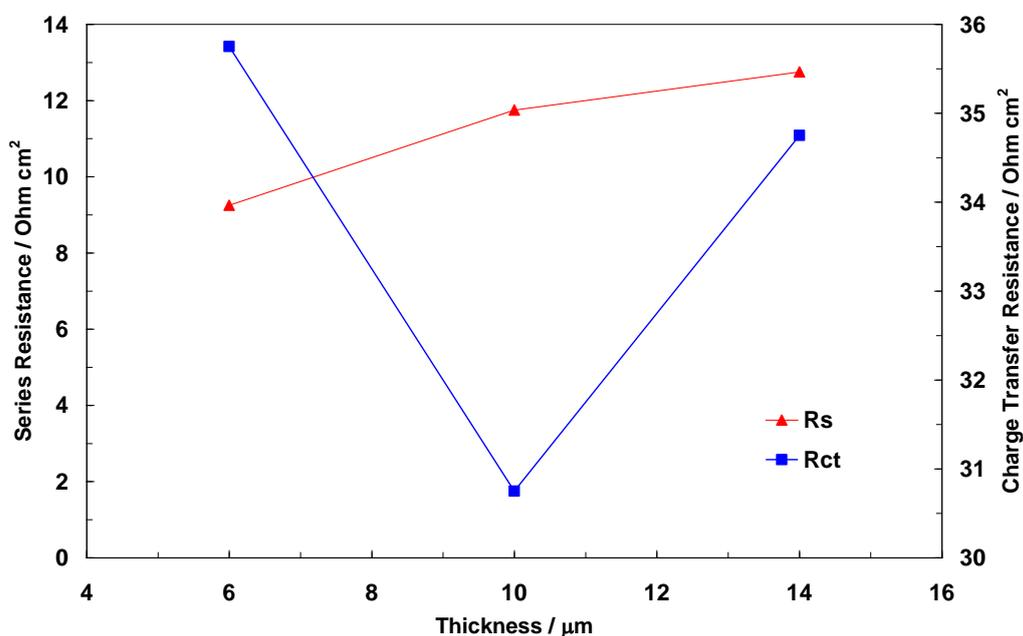
**Figure 7.** Variation of Series (a) and Charge Transfer (b) Resistance as a function of  $\text{TiO}_2$  thickness of the photo-anodes.
