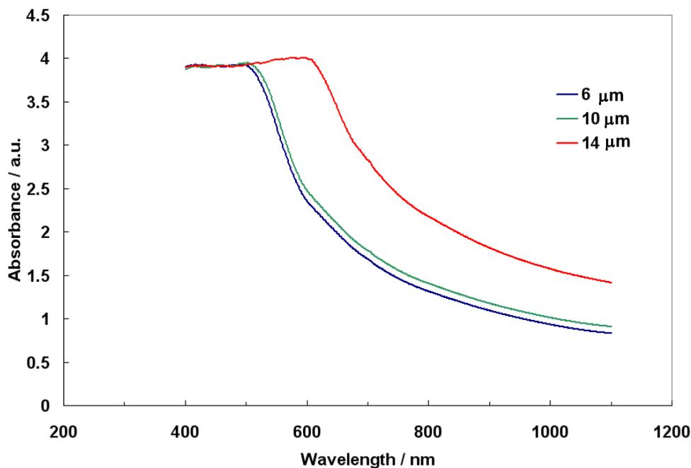
**Figure 4.** Absorbance spectra of the photo-anodes with different thicknesses (6, 10 and 14  $\mu m$ ).
