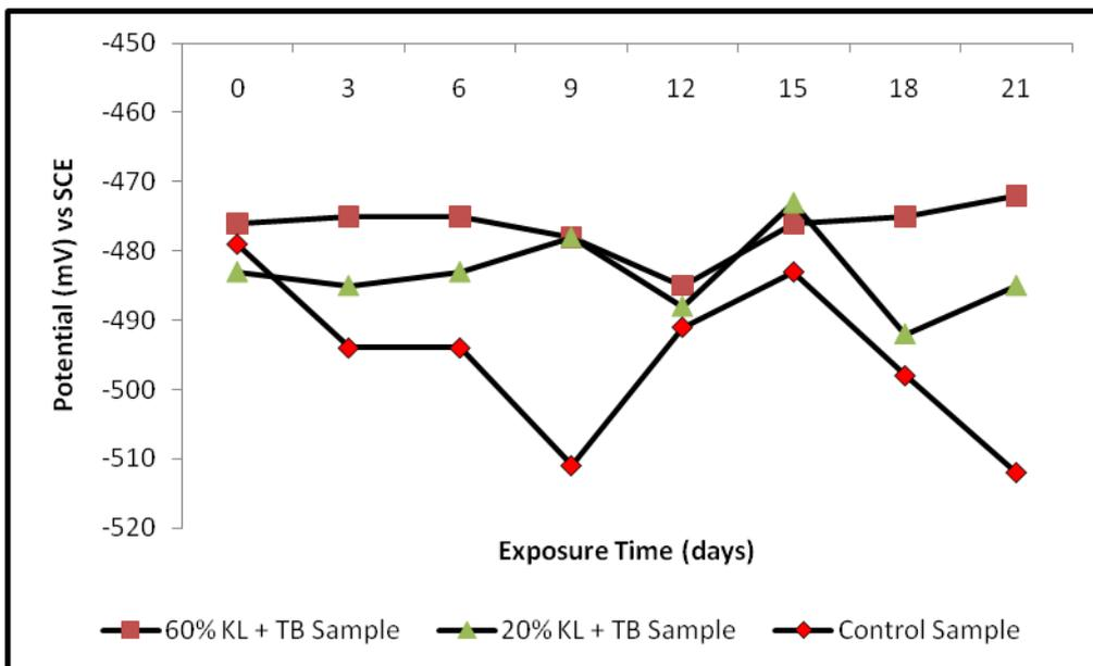
**Figure 8:** Variation of potential with exposure time for the mild steel specimen immersed in acid chloride, with varied percent concentrations of added kola leaf and tobacco extracts. (KL, TB = Kola leaf and tobacco extracts)
