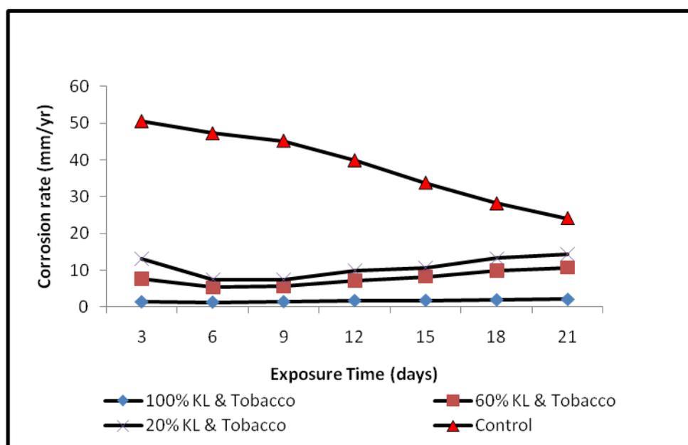
**Figure 4:** Variation of corrosion rate with exposure time for the mild steel specimen immersed in acid chloride, with varied percent concentrations of added kola leaf and tobacco extracts.
