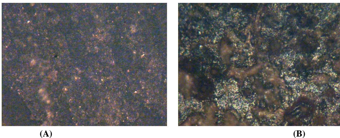
**Figure 11:** Mild steel test specimens: (a) after 21 day immersion in 60% concentrations of added kola leaf and tobacco; and (b) 21 days in 60% concentrations of added kola nut, kola leaf and tobacco extracts respectively.
