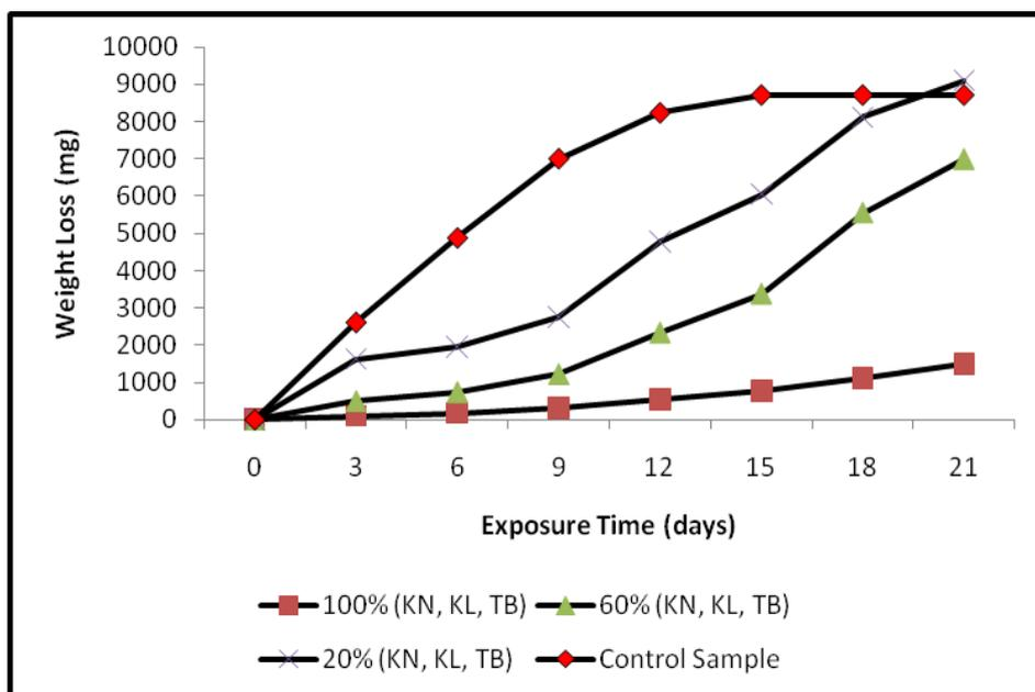
Figure 5: Variation of weight loss with exposure time for the mild steel specimen immersed in acid chloride, with varied percent concentrations of added kola nut, kola leaf and tobacco extracts.
