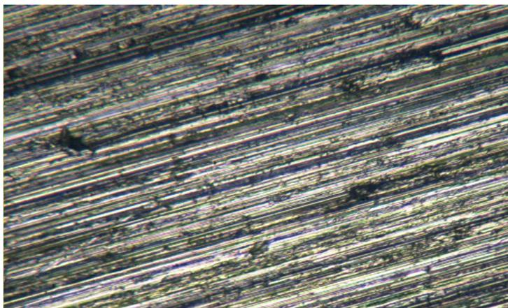
**Figure 12:** Mild steel specimen before immersion
