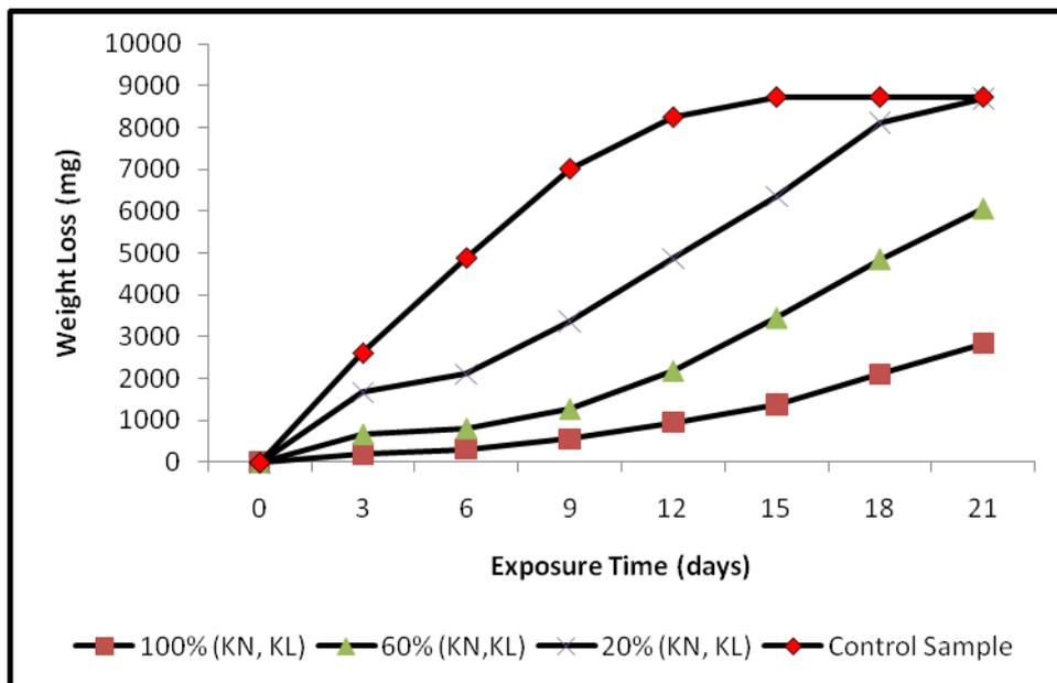
**Figure 1:** Variation of weight loss with exposure time for the mild steel specimen immersed in acid chloride, with varied percent concentrations of added kola nut and kola leaf extracts. (KN, KL = kola nut and kola leaf extracts respectively)
