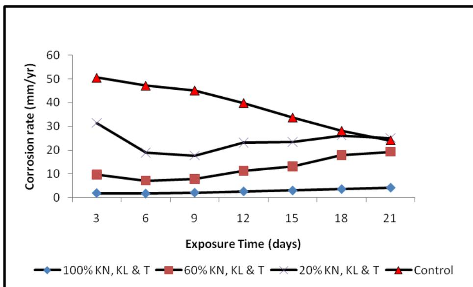
**Figure 6:** Variation of corrosion rate with exposure time for the mild steel specimen immersed in acid chloride, with varied percent concentrations of added kola nut, kola leaf and tobacco extracts.
