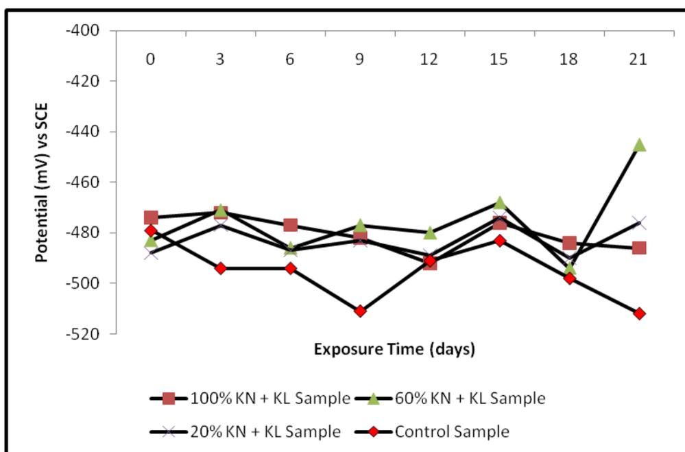
**Figure 7:** Variation of potential with exposure time for the mild steel specimen immersed in acid chloride, with varied percent concentrations of added kola nut and kola leaf extracts. (KN, KL = Kola nut and leaf extract)
