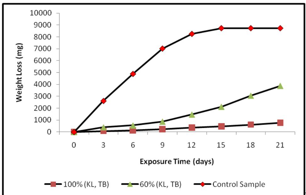
**Figure 3:** Variation of weight loss with exposure time for the mild steel specimen immersed in acid chloride, with varied % concentrations of added kola leaf tobacco extracts.
