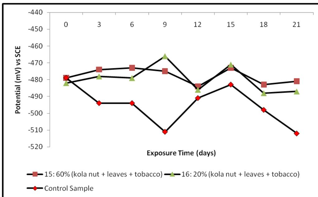
**Figure 9:** Variation of potential with exposure time for the mild steel specimen immersed in acid chloride, with varied percent concentrations of added kola nut, kola leaf and tobacco extracts. (KN, KL, TB = Kola nut, Kola leaf and tobacco extracts)
