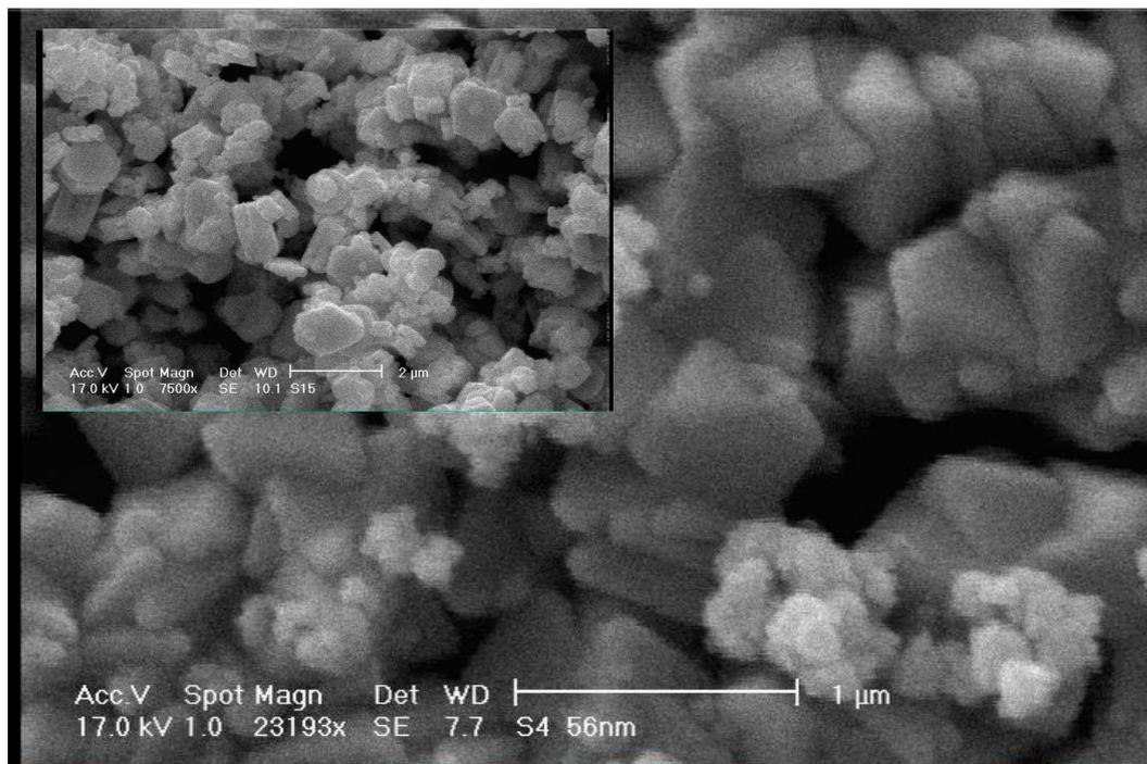
**Figure 1.** SEM image of the electrodeposited cadmium oxide on glassy carbon, scale bare 150 nm. Inset: The SEM image with lower magnification for the same sample, scale bar is 5.0μm.
