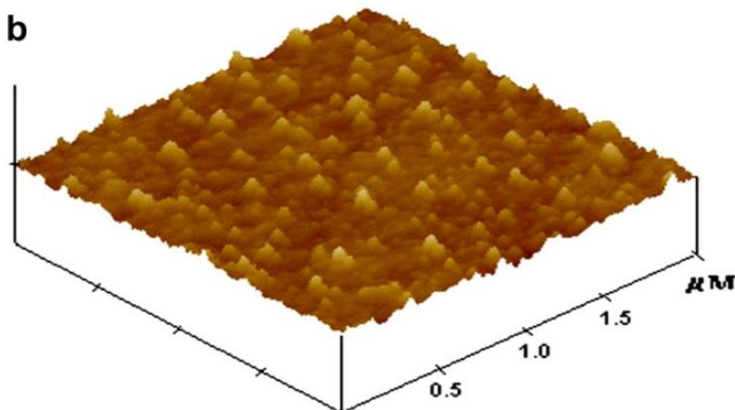
**Figure 2.** AFM images of the GC electrode surface (a) before and (b) after modification with the cadmium oxide film. The images were obtained using tapping mode AFM, and the cadmium oxide film was electrodeposited by cycling the potential once between 1.2 and -1.1V at a scan rate of  $100 \text{ mVs}^{-1}$
