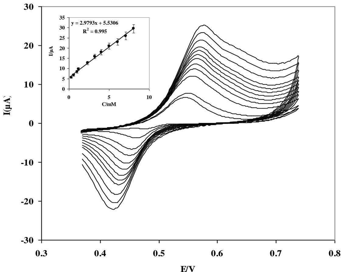
**Figure 4.** Cyclic voltammograms of cadmium oxide nanoparticles modified GC electrode in buffer solution pH 7 at scan rate  $20\text{ mVs}^{-1}$  with increasing PA concentration (from inner to outer) 1,2,3,5,7,10,12,15,20,25,30,35,40,45 and  $50\mu\text{M}$ . Inset: plot of peak current vs. PA concentrations.
