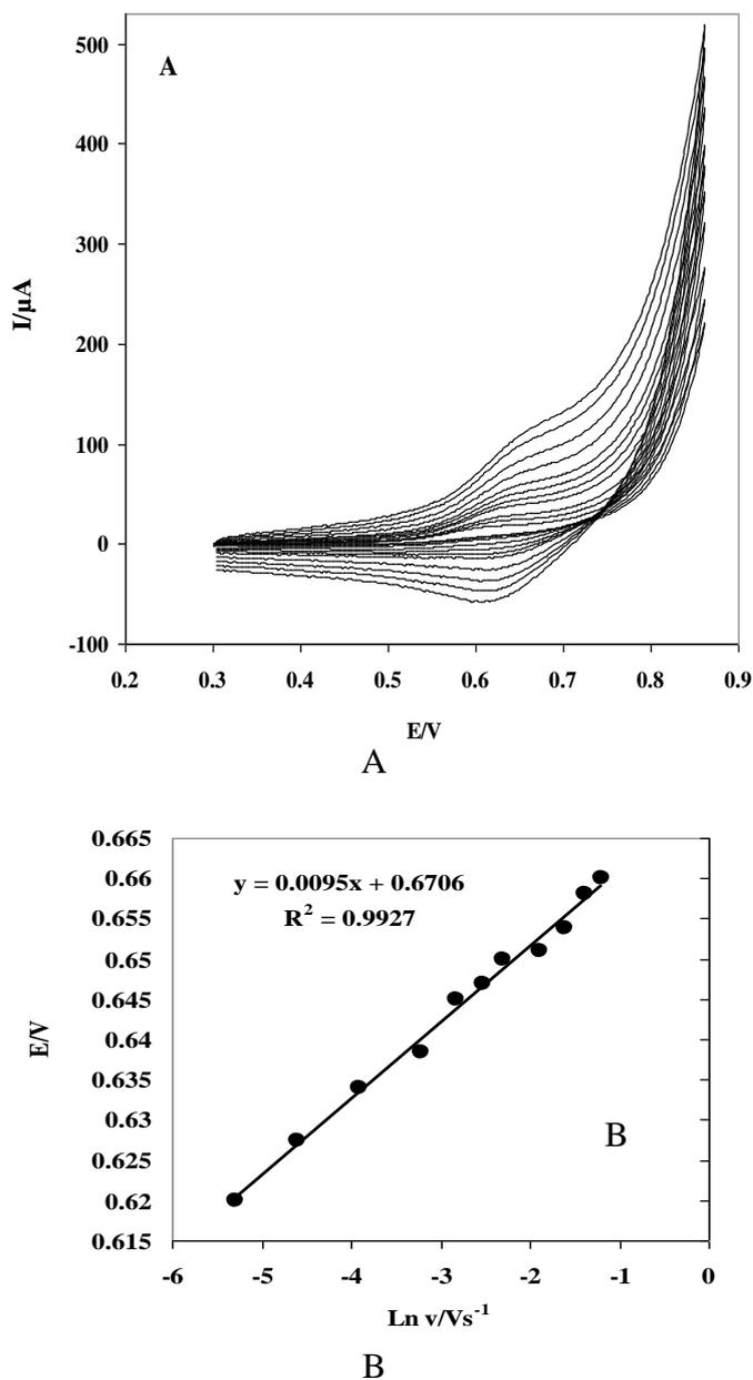
**Figure 5.** (A) Cyclic voltammograms response modified GC electrode in pH 7 buffer solution containing 100  $\mu\text{M}$  of PA at different scan rates (from inner to outer) 10-150  $\text{mVs}^{-1}$ . (B) Plot of  $E_p$  vs.  $\log v$ .
