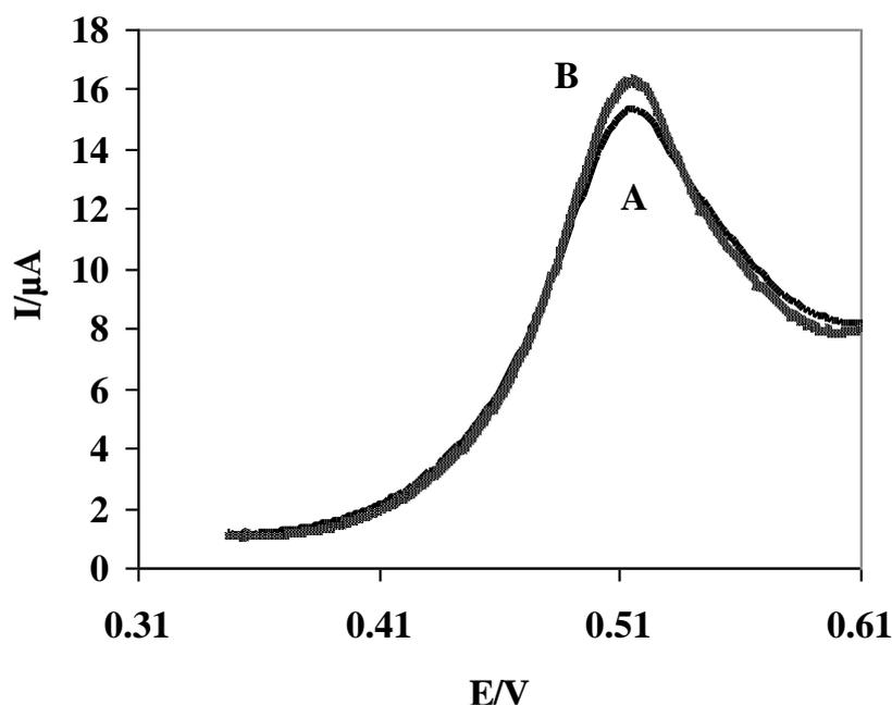
**Figure 7.** Differential pulse voltammograms of a modified electrode in a solution prepared by the addition of 1.00 ml of 0.001 M of PA to; (A) 10.0 ml of pH 7 buffer solution, and (B) 10.0 ml human synthetic serum sample (buffered to pH 7). Pulse amplitude was 50 mV.
