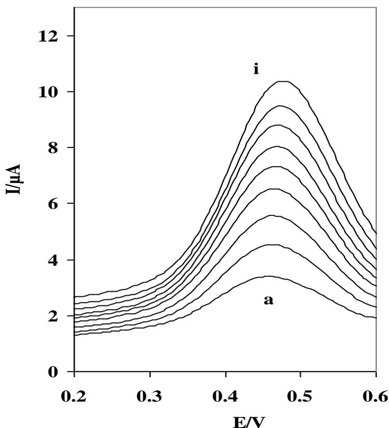
**Figure 6.** Differential pulse voltammograms of PA at the modified electrode with increasing PA concentration 1,3,5,10,20,30,40 and 50  $\mu\text{M}$  PA in pH 7 buffered solutions. Pulse amplitude was 50 mV.
