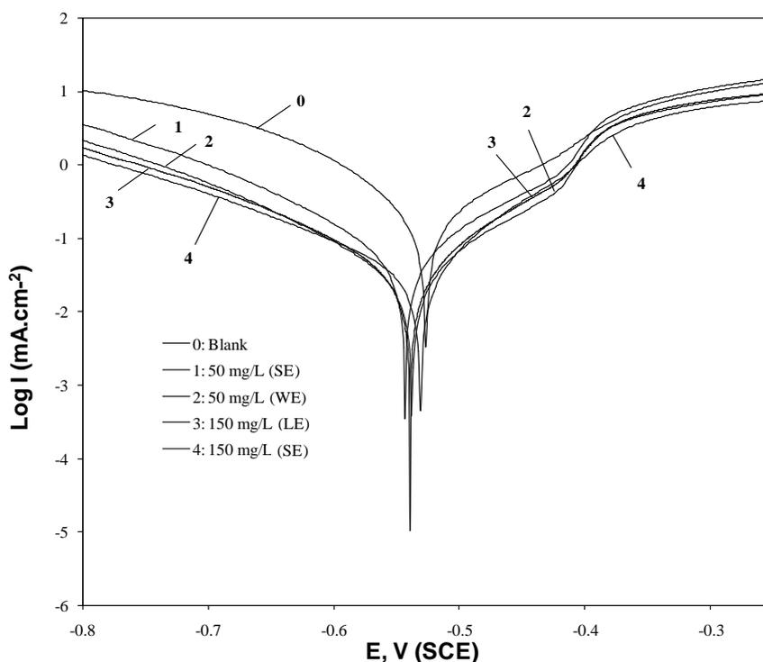
**Figure 2.** Potentiodynamic polarization curves for low carbon steel in 0.1 M HCl containing two concentrations of alkaloids extract from the leaves (LE) and the stems (SE).
