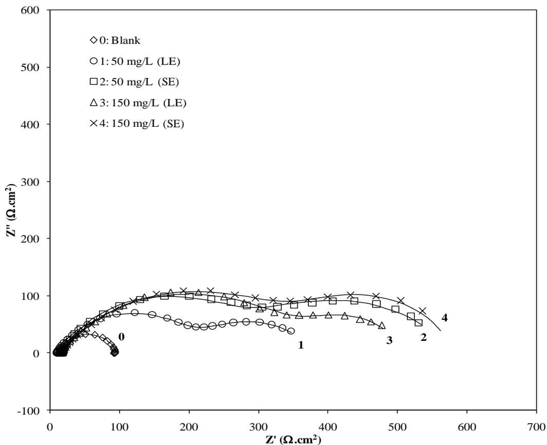
**Figure 3.** Nyquist plots for low carbon steel in 0.1 M HCl solutions in the absence and presence of two concentrations of alkaloids extract from the leaves (LE) and the stems (SE) obtained from experimental and fit data.
