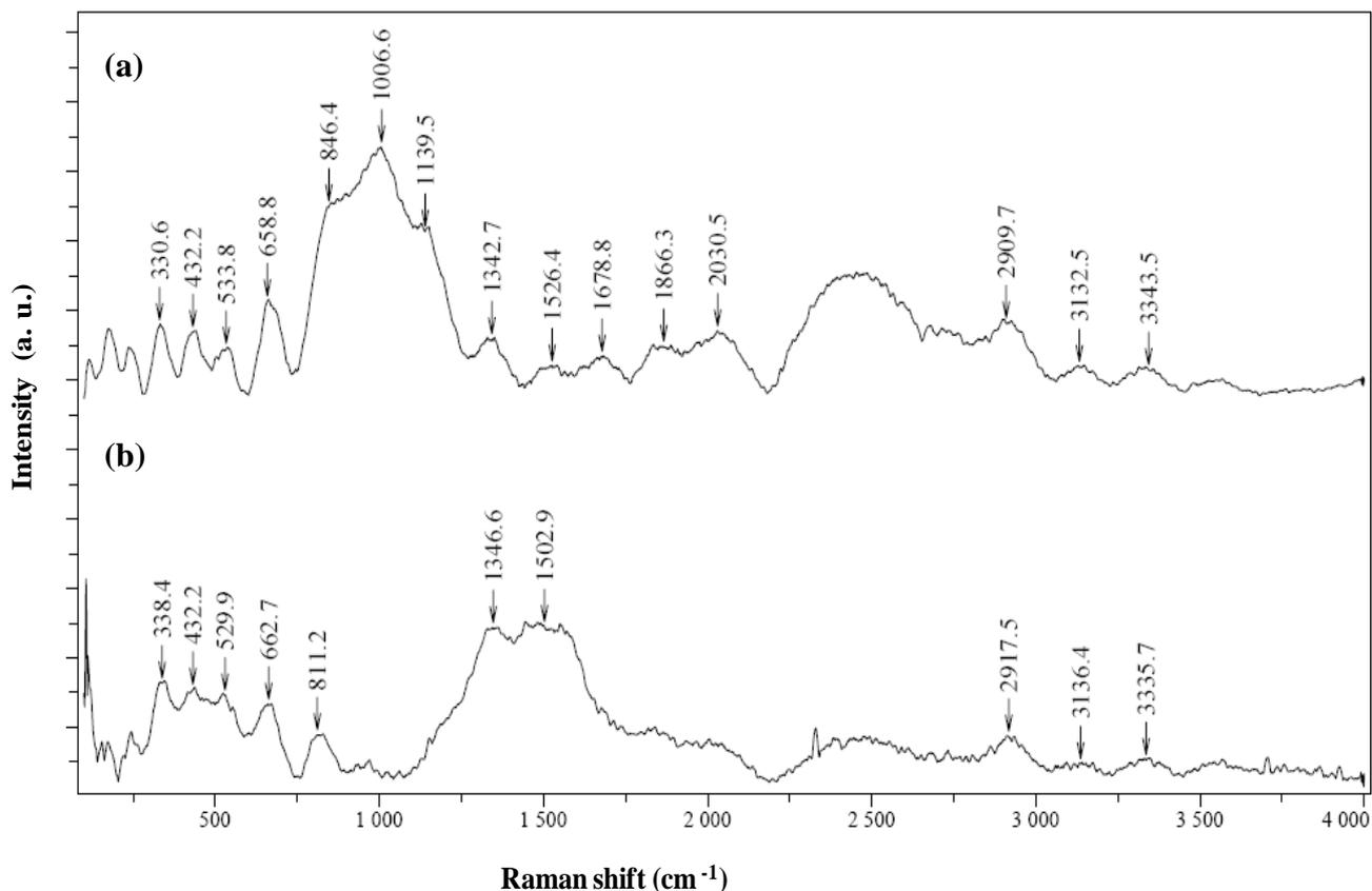
**Figure 9.** Raman spectra obtained for; (a) the solid alkaloids extract; (b) the low carbon steel surface after 3 hours of immersion in 0.1 M HCl + 150 mg/L plant extract.
