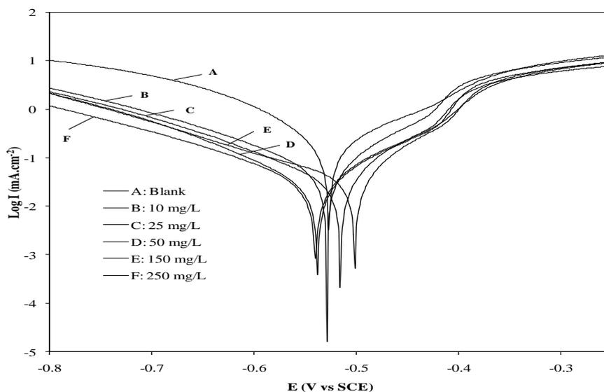
**Figure 6.** Potentiodynamic polarization curves for low carbon steel in 0.1 M HCl solutions containing different concentrations of stems alkaloids extract from *S. guianensis*.
