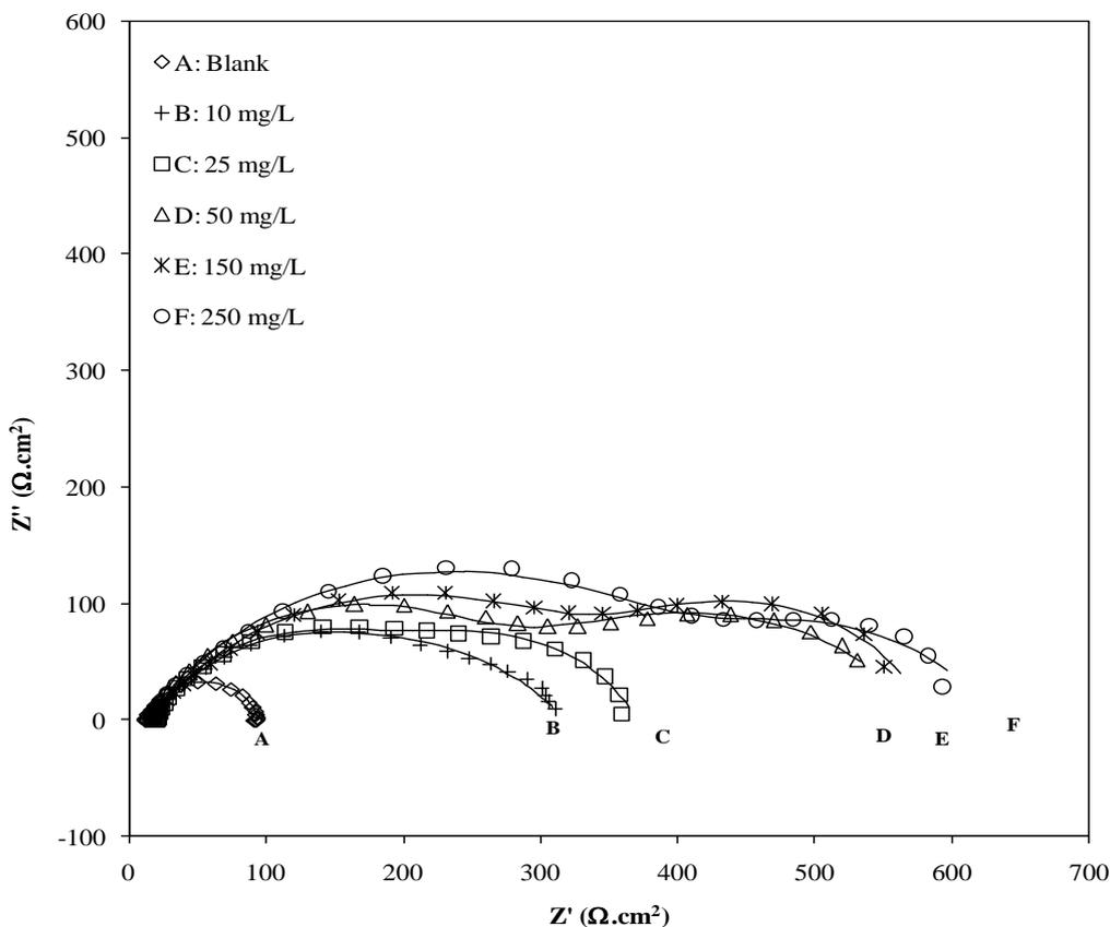
**Figure 7.** Nyquist plots for low carbon steel in HCl solutions with pH 1 in the absence and presence of different concentrations of alkaloids stems extract from *S. guianensis* and the relative fit obtained with the circuit model of Fig. 5.
