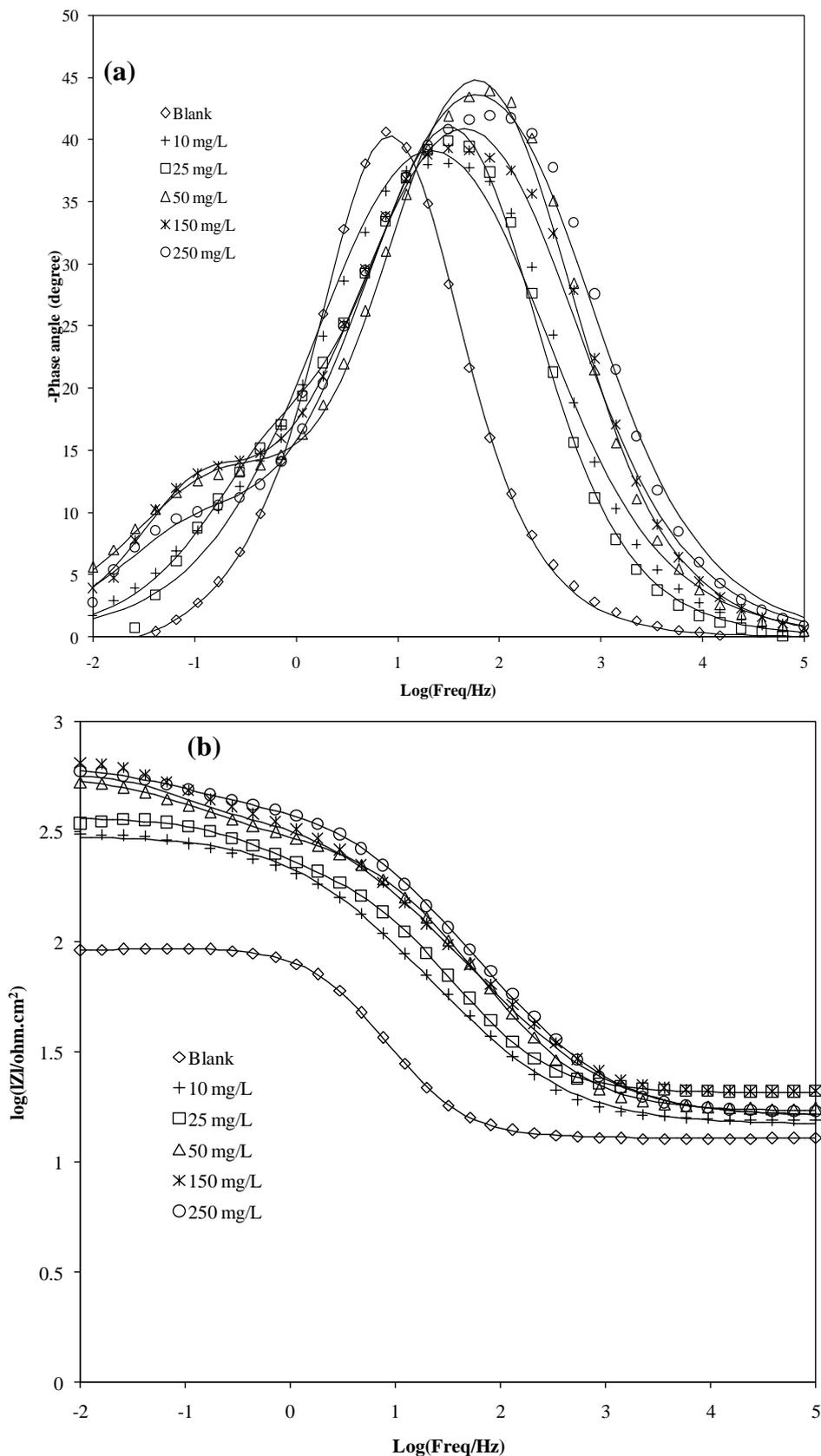
**Figure 8.** The experimental data in the Bode format obtained for low carbon steel in 0.1 HCl at 25°C without and with various concentrations of stems alkaloids extracts and the relative fit obtained with the circuit model of Fig. 5.
