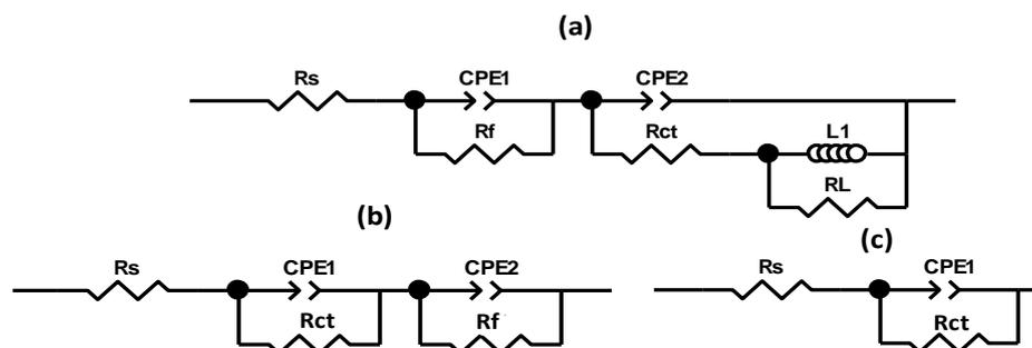
**Figure 5.** The equivalent circuit model used to fit the impedance data for low carbon steel in the absence; (a) and the presence of alkaloids extracts; (b) (c).
