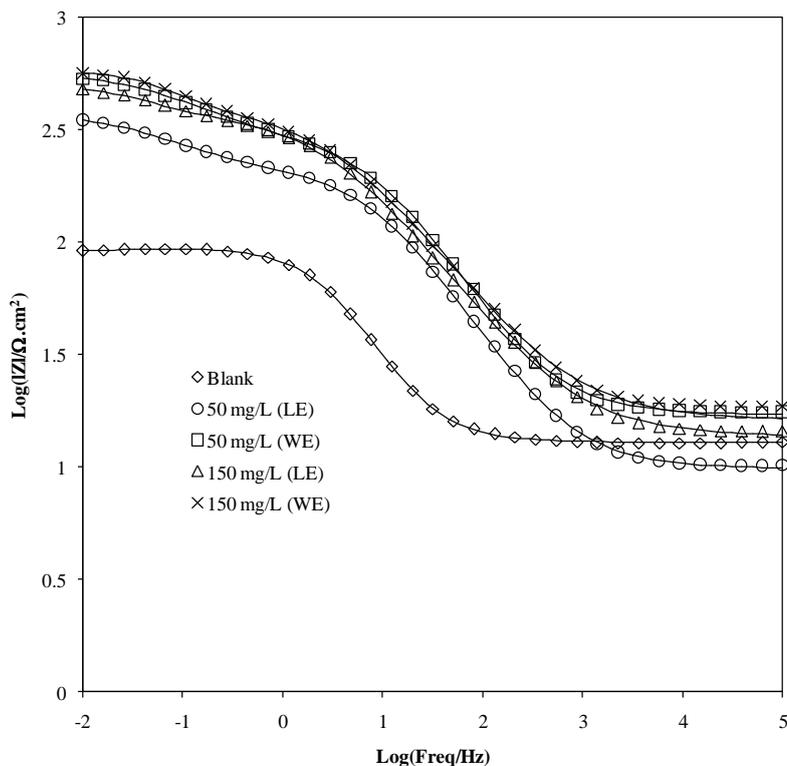
**Figure 4.** The experimental data in the Bode format obtained for low carbon steel in 0.1 M HCl solutions at 25°C without and with two concentrations of alkaloids extract from the leaves (LE) and the stems (SE) and the relative fit obtained with the circuit model of Fig. 5.
