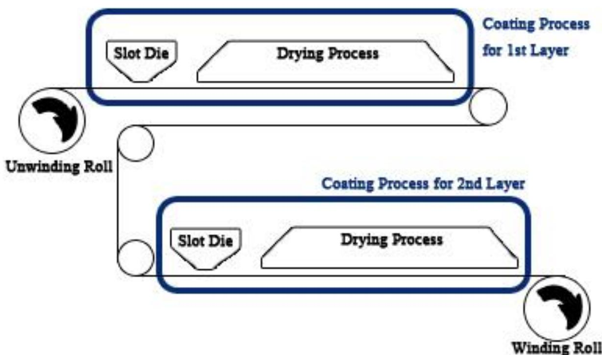
Figure 1. Schematic of Roll-to-Roll System with Drying Process
