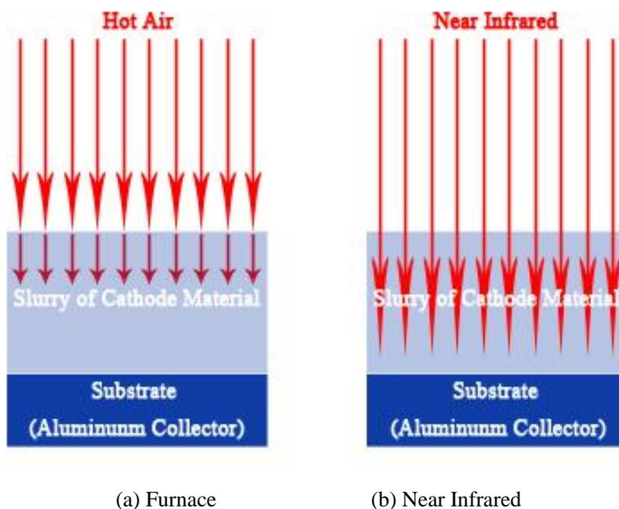
**Figure 2.** Heat Transfer Mechanisms
