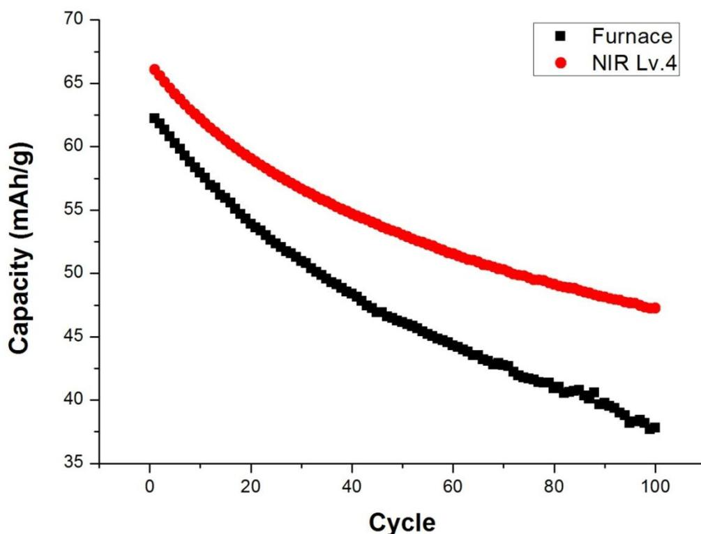
**Figure 3.** Life Cycles of Lithium Ion battery using Thin Film Electrode dried by Furnace and NIR
