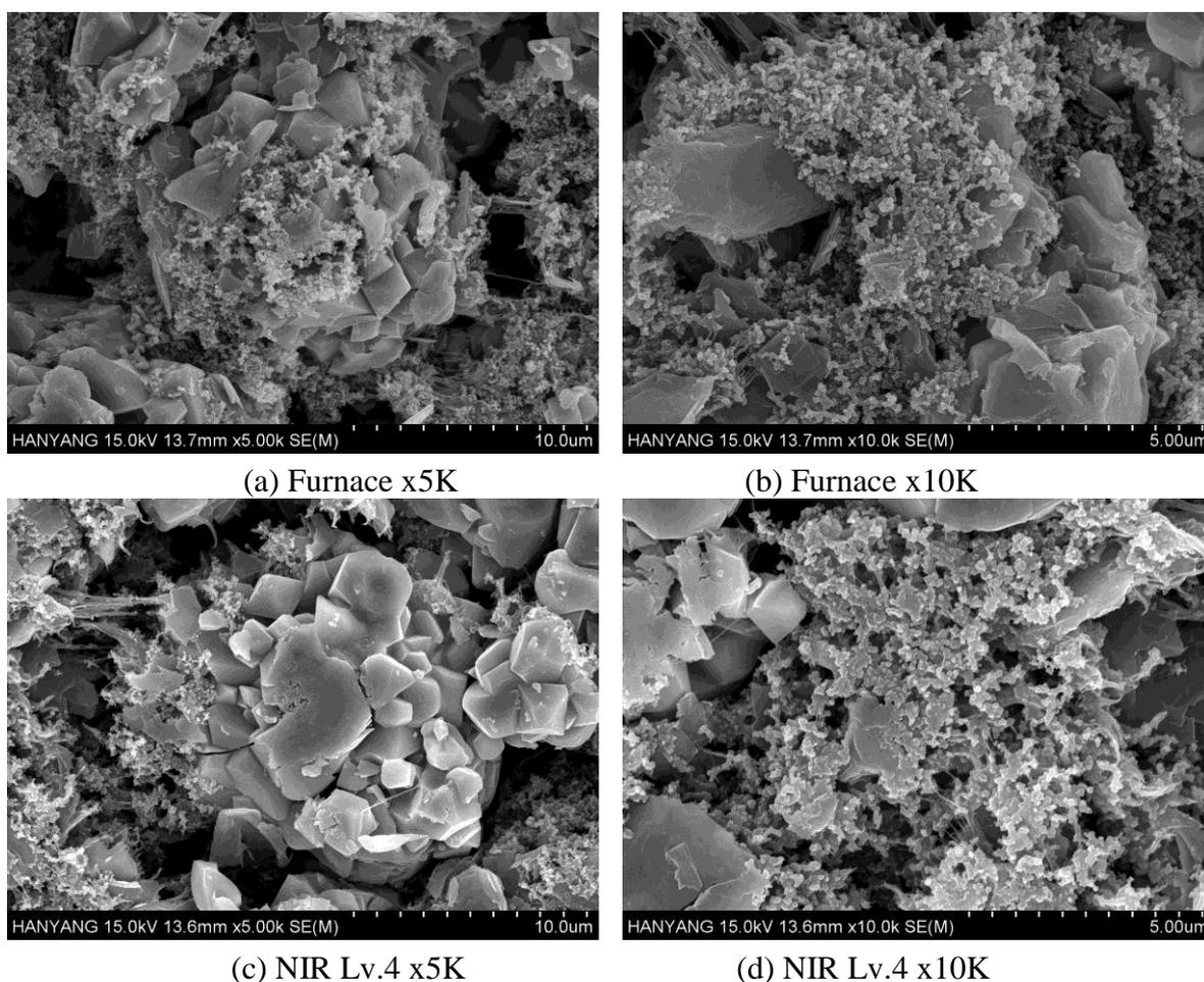
Figure 5. SEM Images of Spinel Type  $\text{LiMn}_2\text{O}_4$  Thin Film Electrode
