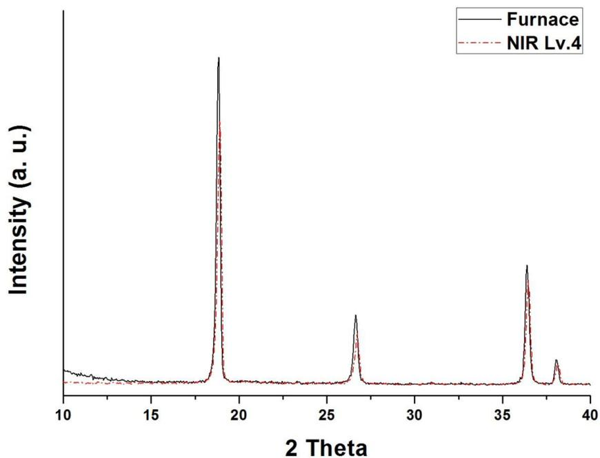
**Figure 4.** Result of XRD of Spinel Type LiMn<sub>2</sub>O<sub>4</sub> Thin Film Electrode
