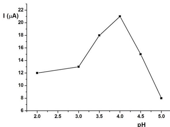
**Figure 5.** Effect of pH on peak current: accumulation potential -1.4 V, accumulation time 120s.
