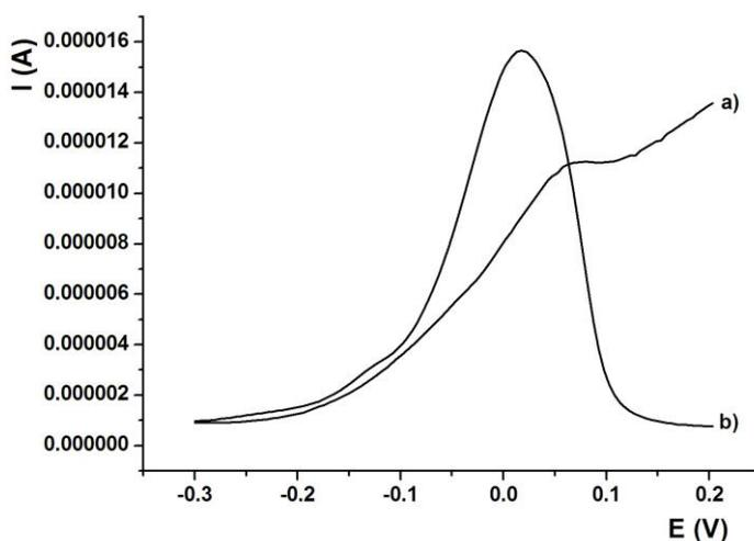
**Figure 4.** Pulse anodic stripping voltamogram of  $2 \mu\text{M}$  of Cu at bare glassy carbon electrode (a) and modified electrode (b); electrolyte acetic buffer pH 4, accumulation potential  $-1.4 \text{ V}$ , accumulation time 120s.
