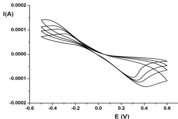
**Figure 2.** Cyclic voltammogram of Cu solution with modified electrode: concentration of Cu was  $1 \times 10^{-5}$ , scan rate  $50 \text{ mVs}^{-1}$ , supporting electrolyte was acetic buffer
