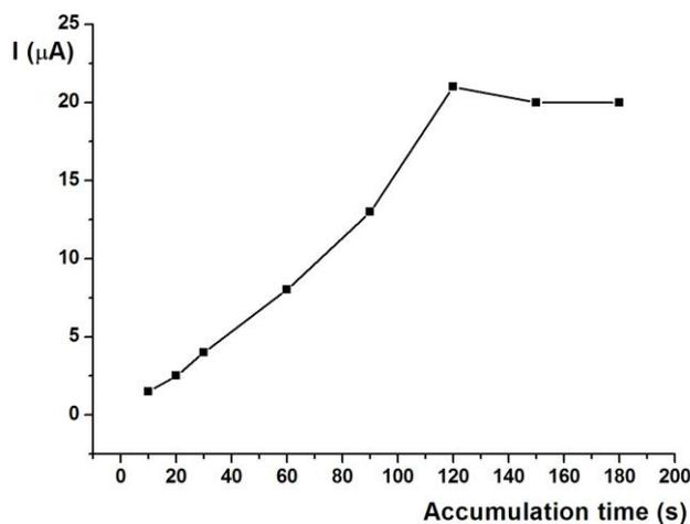
**Figure 6.** Effect of accumulation time on peak current; electrolyte acetic buffer pH 4, accumulation potential -1.4 V
