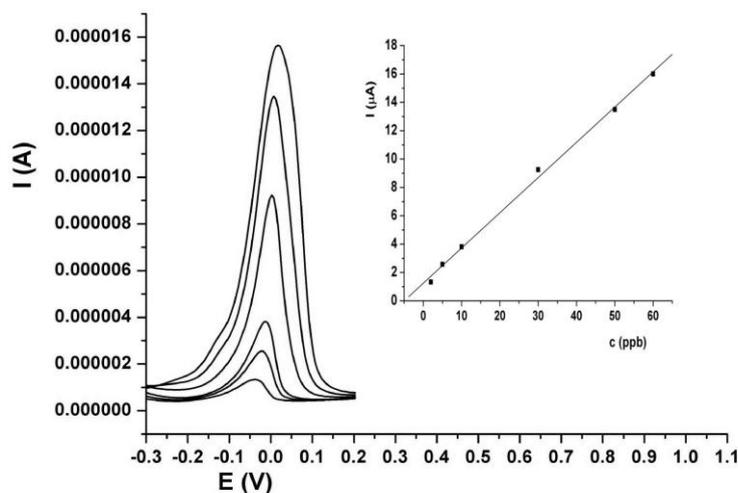
**Figure 7.** DPASV and calibration curve for different concentration of Cu at optimized parameters
