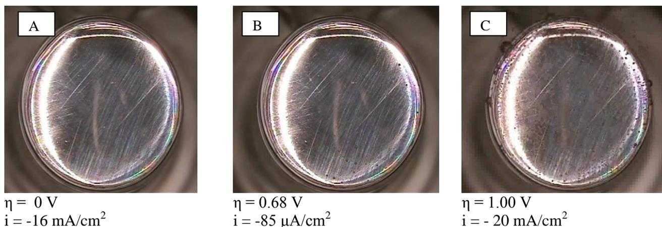
**Figure 7.** Images of nickel surface during the cathodic curve at 25 °C in 992 g/l LiBr at different overpotentials.
