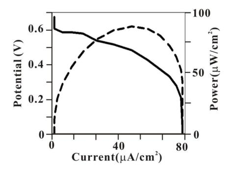
**Figure 5**. Polarization curve (solid line) and dependence of the power density on the operating voltage (dashed line) for a biofuel cell consisting of MWCNTs/GOx modified electrode as anode in combination with a PtNPs/laccase electrode as cathode. As fuel a 5 mM solution of glucose in PBS (pH 7.0) containing 1 mM ABTS was used.
