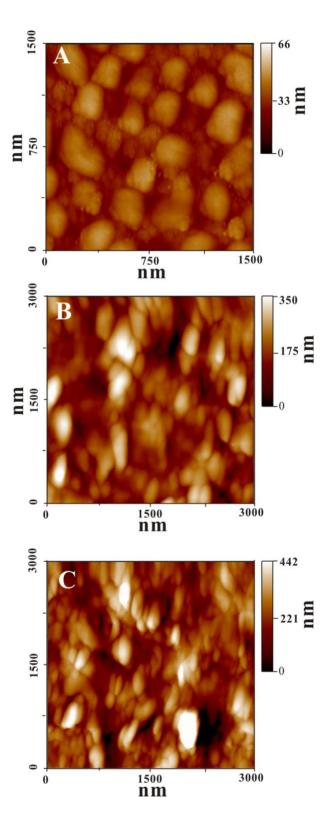
Figure 1. AFM images of (A) PtNPs; (B) only laccase; (D) PtNPs /laccase on ITO electrode.
