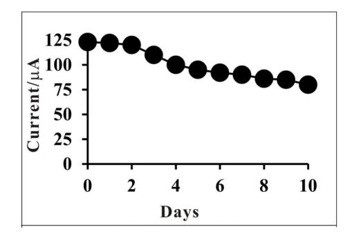
**Figure 4**. Reduction oxygen peak current of PtNPs/laccase modified electrodes stored in pH 7.0 PBS at 4 °C for 10 consecutive days.
