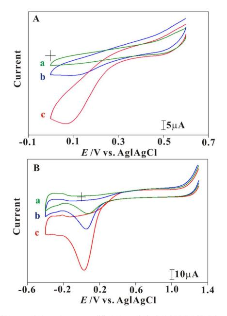
**Figure 2.** (A) CVs recorded at a laccase modified electrode in 0.1M PBS (pH 7.0 containing 1 mM ABTS) saturated with nitrogen (curve a), ambient air (curve b) and oxygen (curve c). Scan rate 100 mVs<sup>-1</sup> in the potential range of 0.6 to 0 V. (B) CVs recorded at a PtNPs modified electrode in 0.1M PBS (pH 7.0 containing 1 mM ABTS) saturated with nitrogen (curve a), ambient air (curve b) and oxygen (curve c). Scan rate 100 mVs<sup>-1</sup> in the potential range of 1.3 to -0.4 V.
